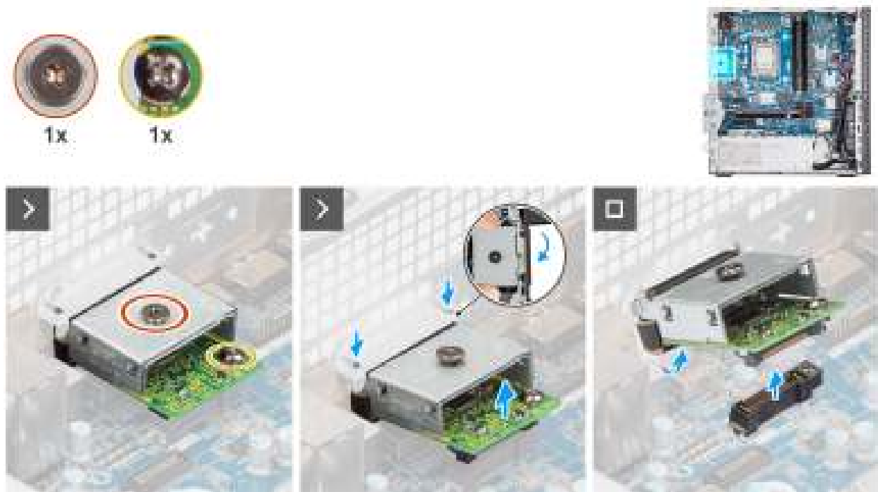
Figure 76. Removing the optional DisplayPort module
