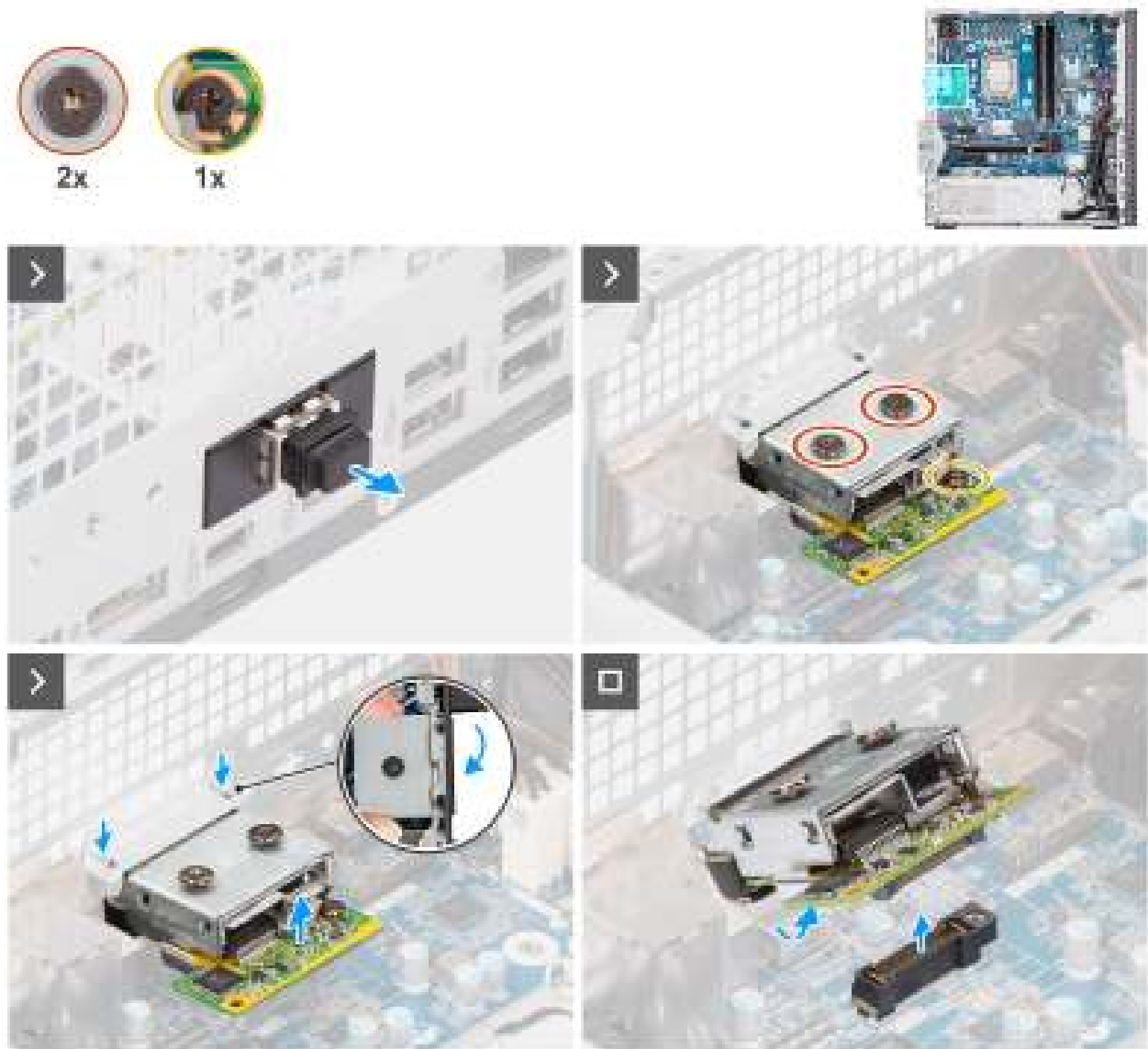
Figure 79. Removing the optional 5GbE Optical module
