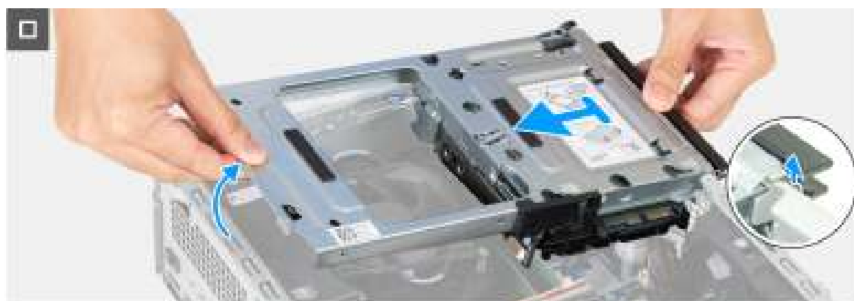
Figure 22. Removing the drive bay
