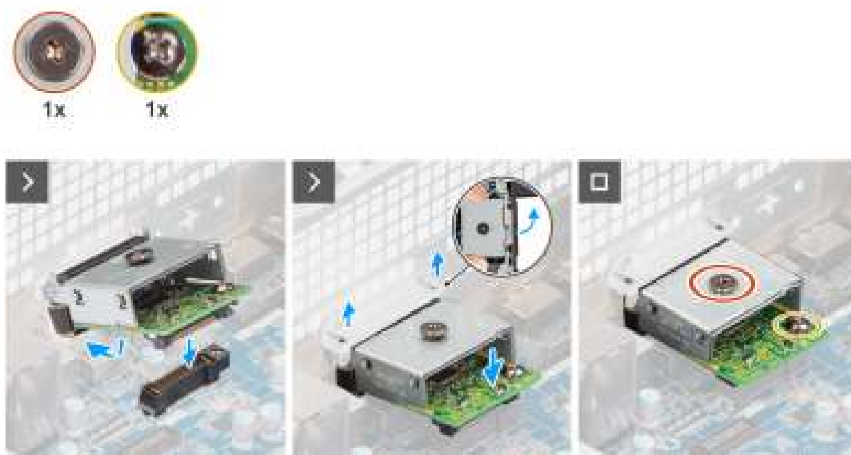
Figure 78. Installing the optional DisplayPort module
