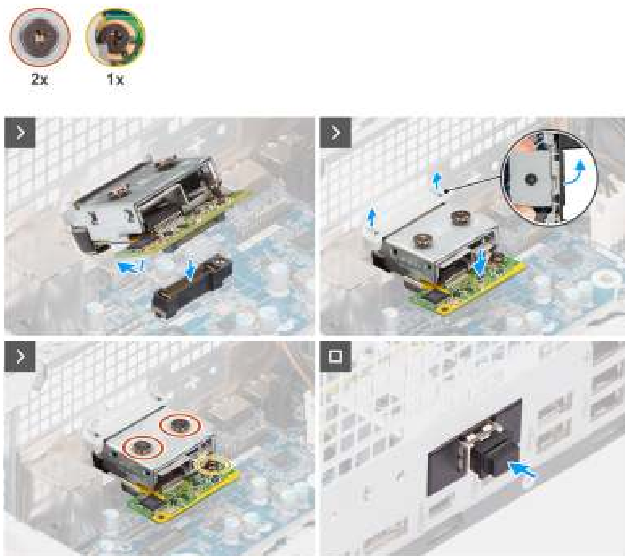
Figure 81. Installing the optional 5GbE Optical module
