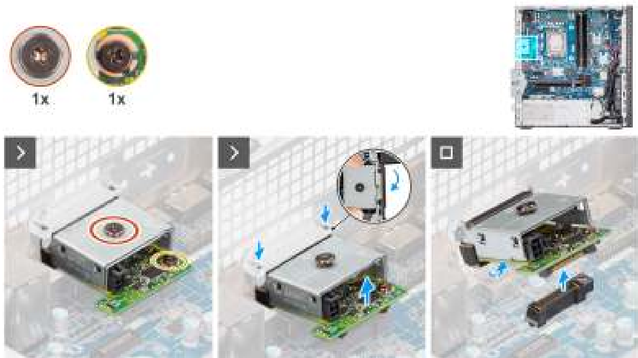
Figure 67. Removing the optional Thunderbolt module
