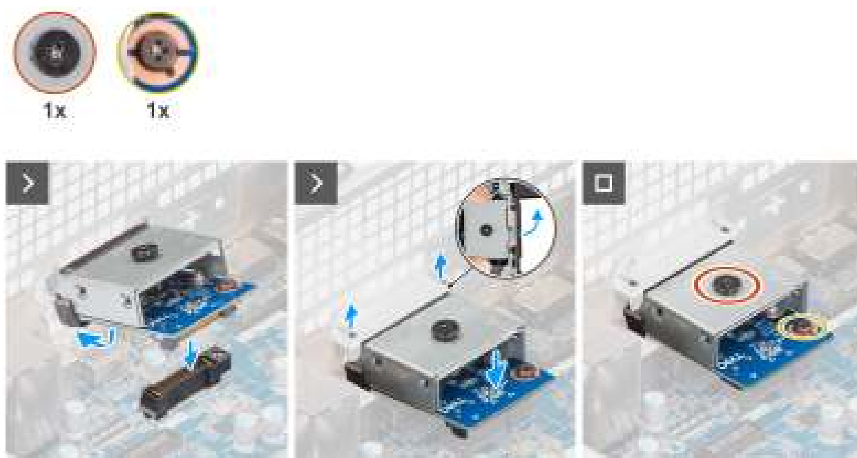
Figure 63. Installing the optional VGA module
