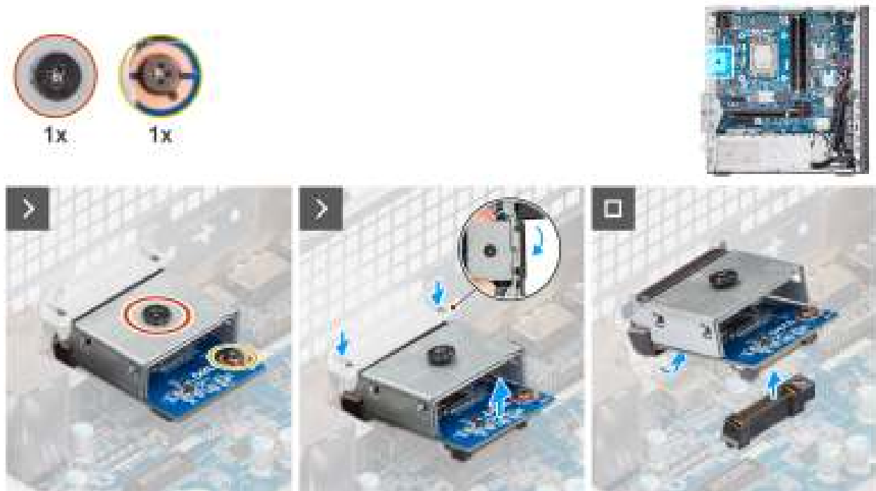
Figure 73. Removing the optional HDMI module
