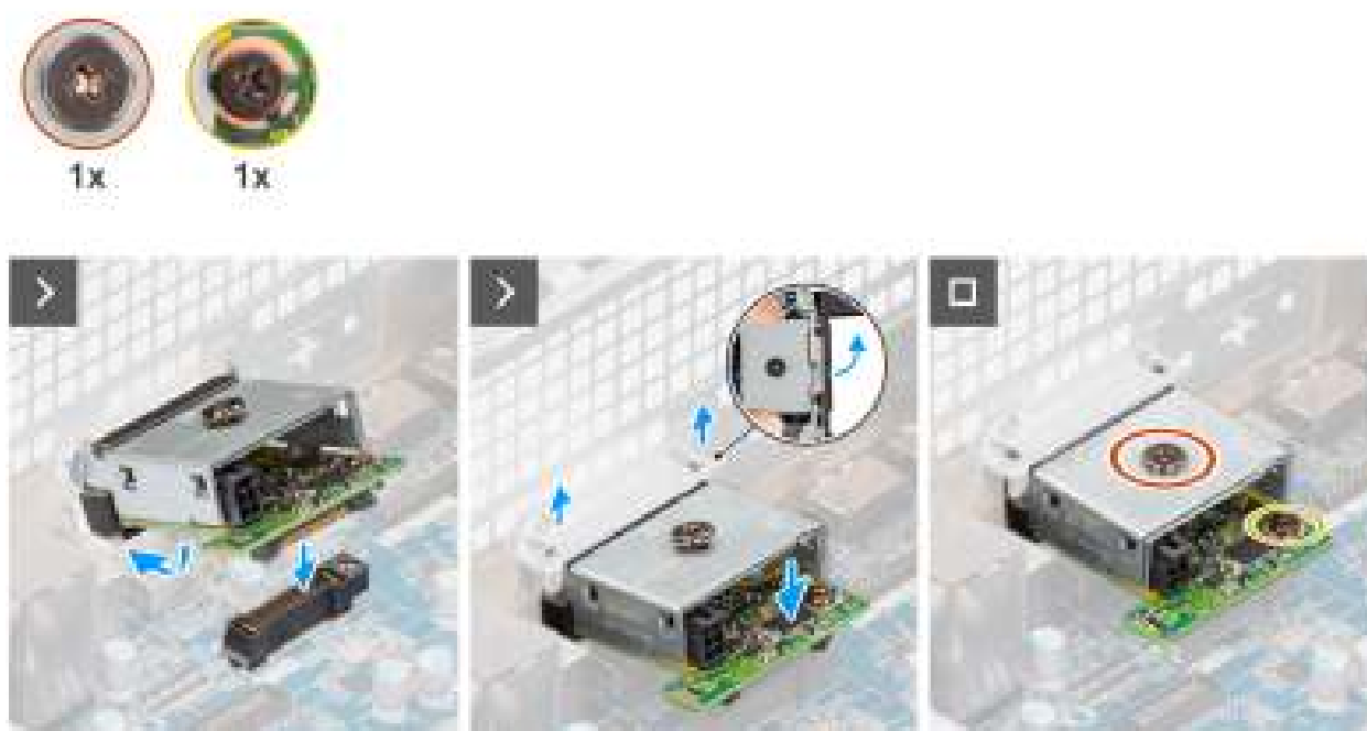
Figure 69. Installing the optional Thunderbolt module
