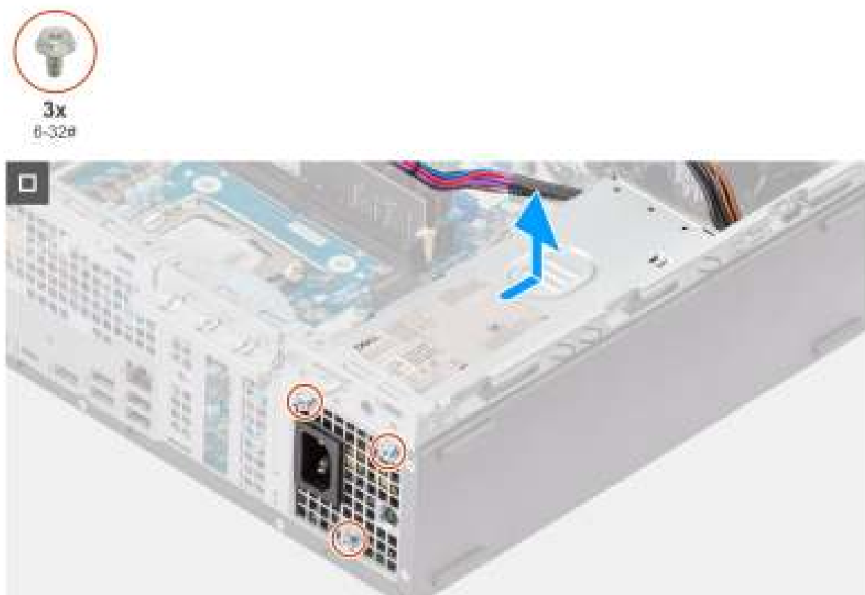
Figure 58. Installing the power-supply unit
