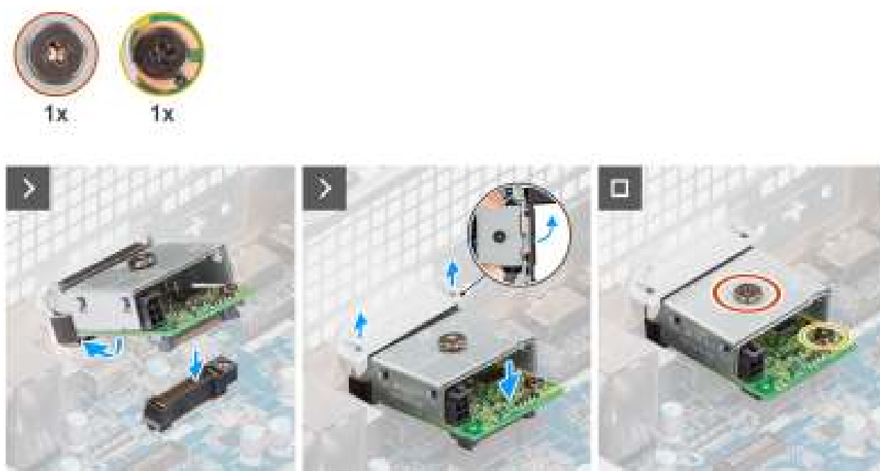
Figure 66. Installing the optional USB module
