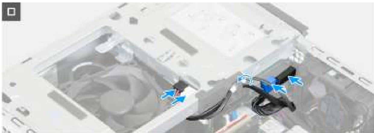
Figure 24. Installing the drive bay
