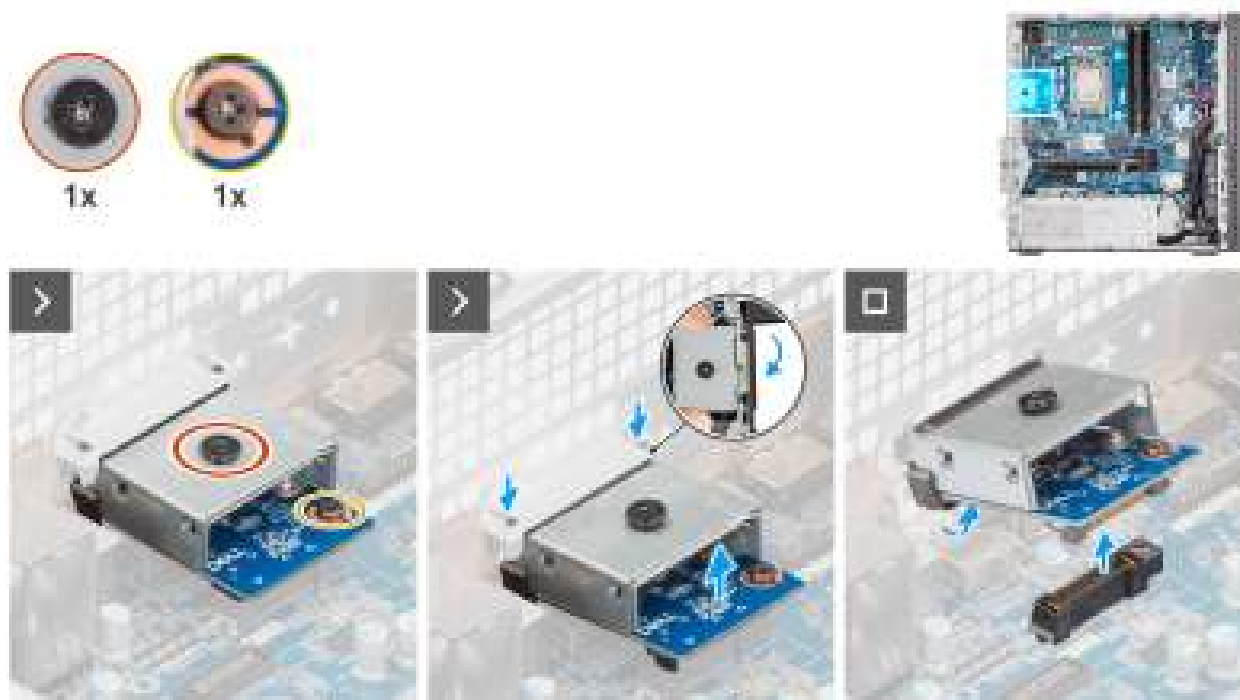
Figure 61. Removing the optional VGA module
