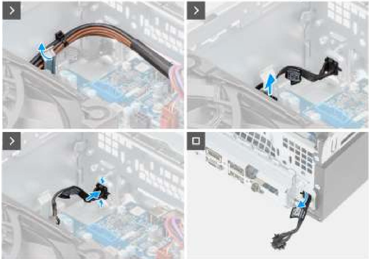
Figure 45. Removing the power button
