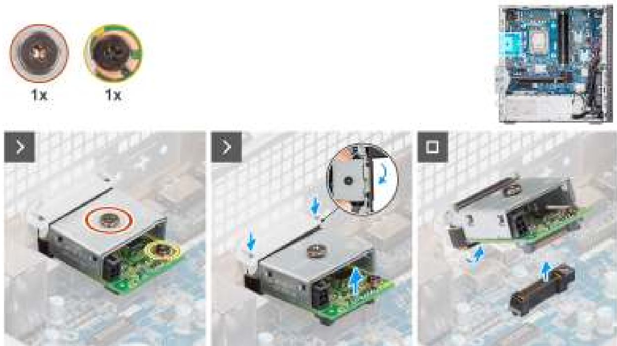
Figure 64. Removing the optional USB module
