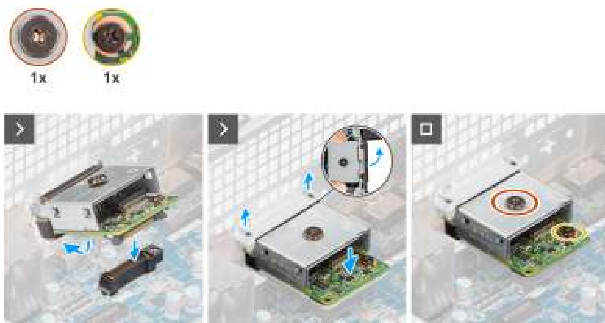
Figure 72. Installing the optional LAN module
