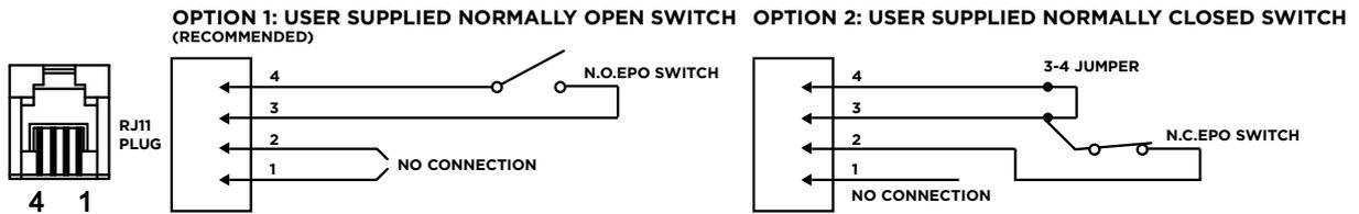
3. After wiring, make sure the external EPO/ROO switch is not activated to enable UPS output.
