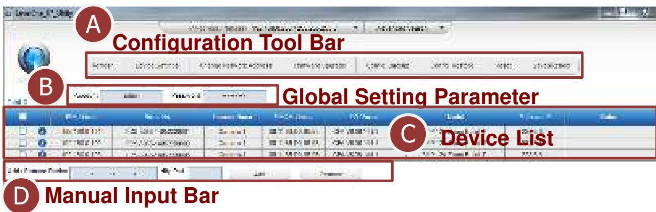
5. To access the device, simply use the mouse to click on the IP address on the device list. This will initiate the Internet Explorer to allow user to access the device's firmware.
