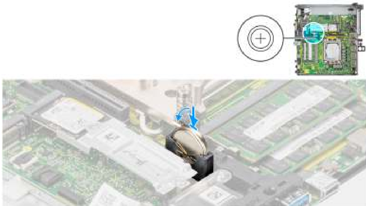
Figure 9. Installation de la pile bouton
