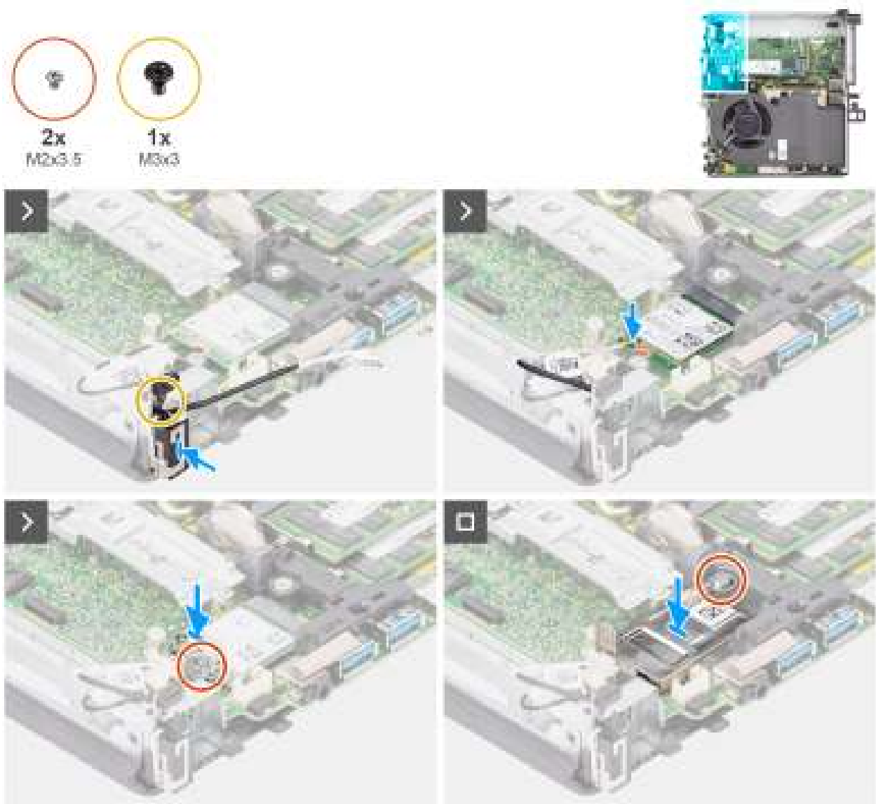
Figure 53. Installation de l'antenne interne (emplacement 1)
