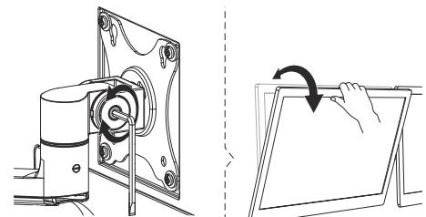
Note: If the display does not stop at your desired position, tighten the screw as shown.
