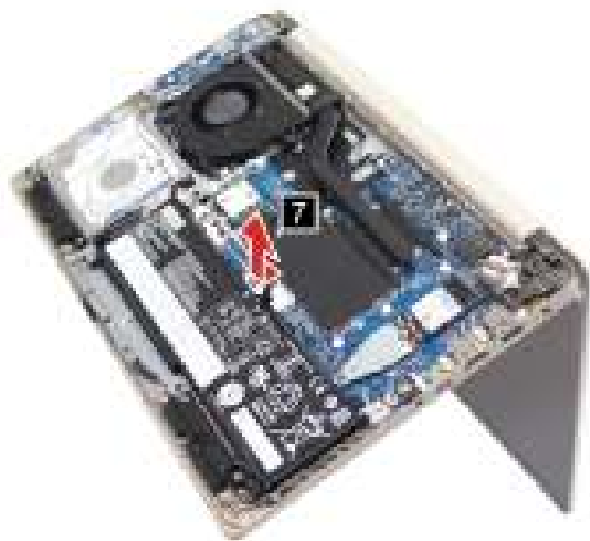
Figure 56. Remove the upper case assembly
