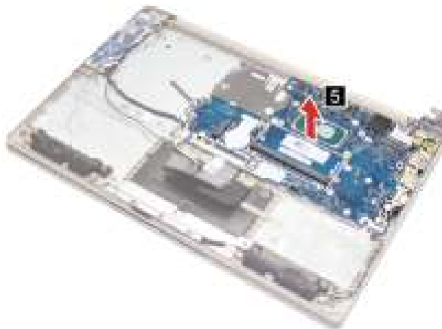
Figure 47. Remove the system board
