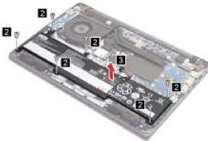
Figure 18. Remove the battery pack
