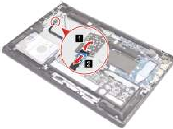
Figure 43. Disconnect the battery pack cable
