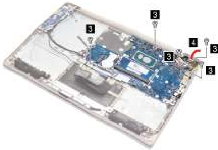
Figure 46. Remove five screws and open the right hinge
