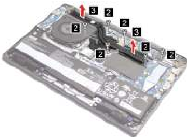
Figure 26. Loosen six screws and remove the heat sink
