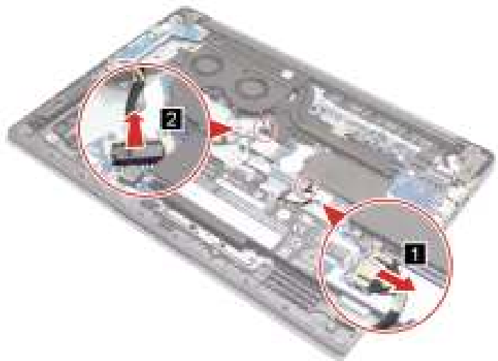
Figure 30. Disconnect the fan cable
