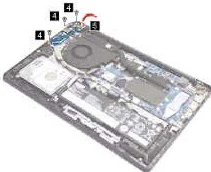
Figure 36. Remove the USB board
