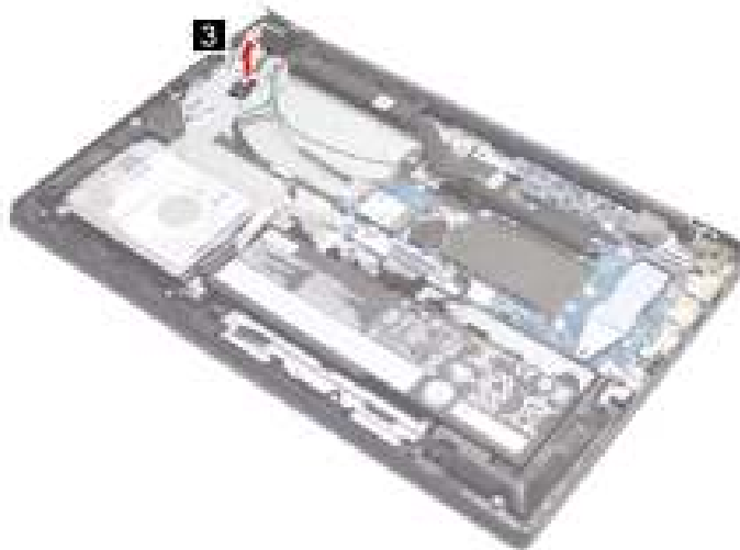
Figure 44. Remove the fingerprint reader
