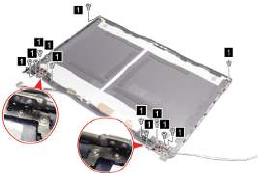
Figure 61. Remove ten screws
