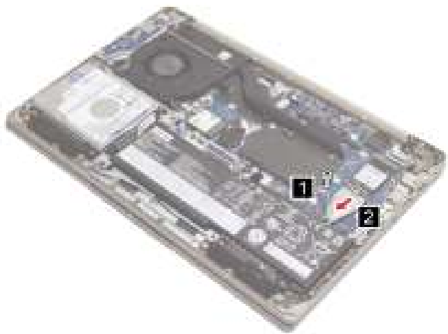
Figure 19. Remove the solid-state drive bracket
