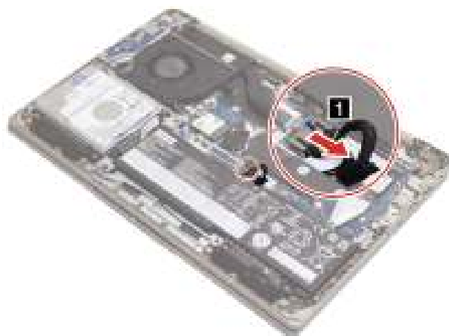
Figure 21. Disconnect the battery pack cable
