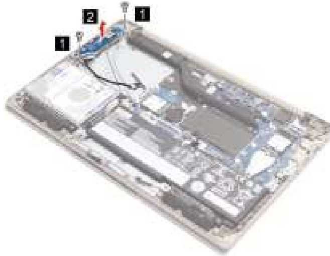
Figure 34. Remove the left I/O board bracket
