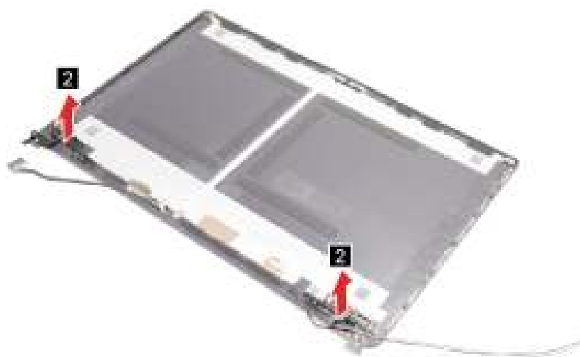
Figure 62. Remove the two hinges
