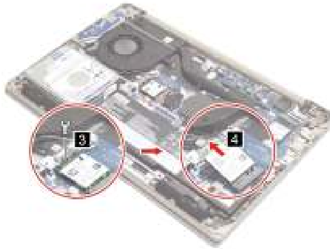
Figure 33. Remove one screw and the Wi-Fi card
