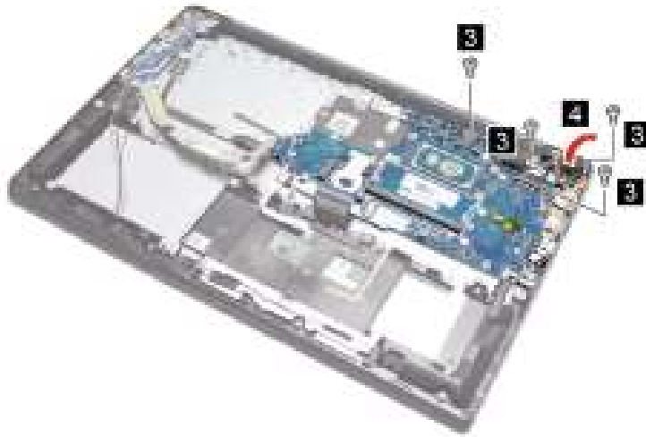
Figure 49. Remove four screws and open the right hinge
