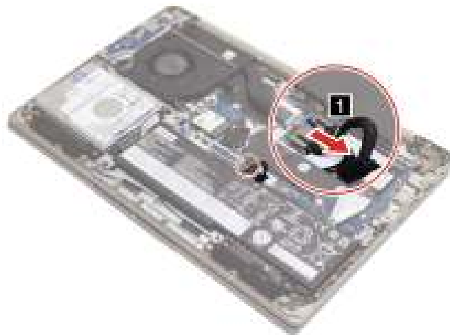
Figure 23. Disconnect the battery pack cable
