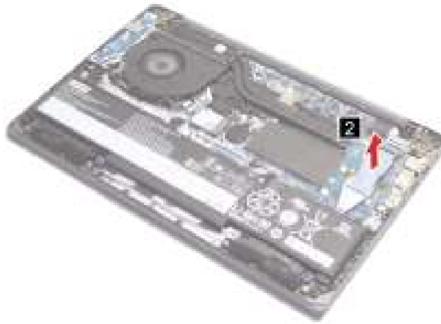
Figure 22. Remove the solid-state drive thermal pad
