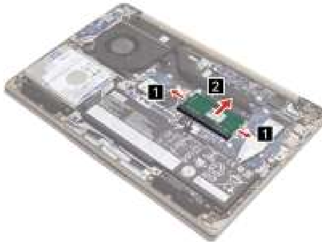
Figure 8. Remove the memory module
