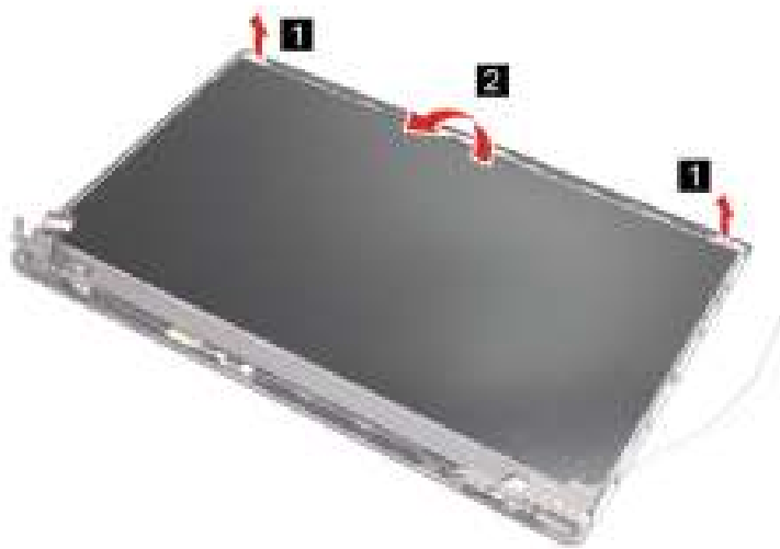
Figure 63. Lift the LCD panel
