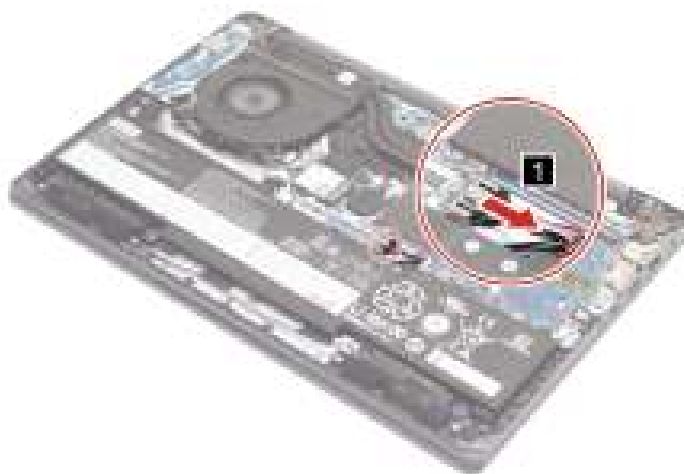
Figure 25. Disconnect the battery pack cable
