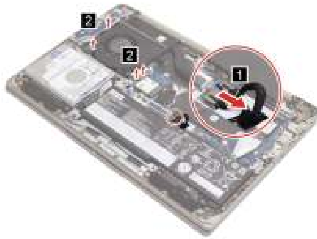
Figure 27. Disconnect the battery pack cable
