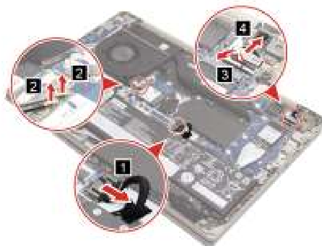
Figure 54. Disconnect the battery pack cable, EDP cables, and antenna cables
