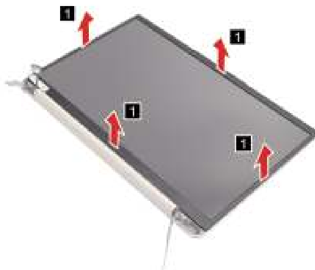
Figure 57. Remove the LCD bezel
