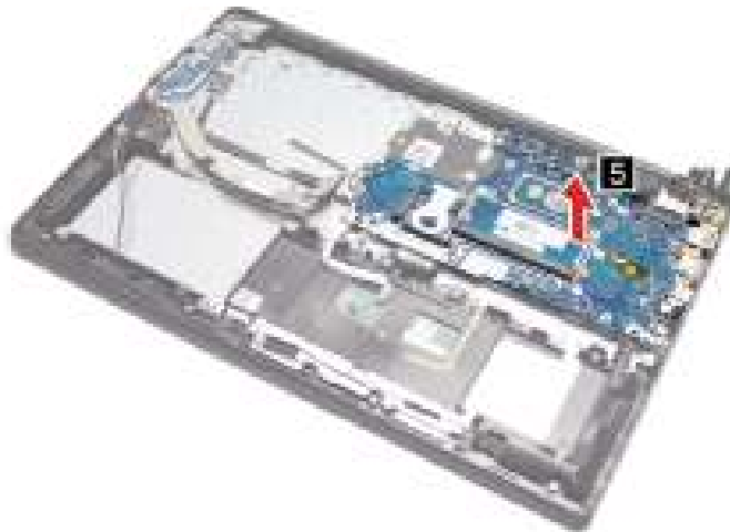
Figure 50. Remove the system board
