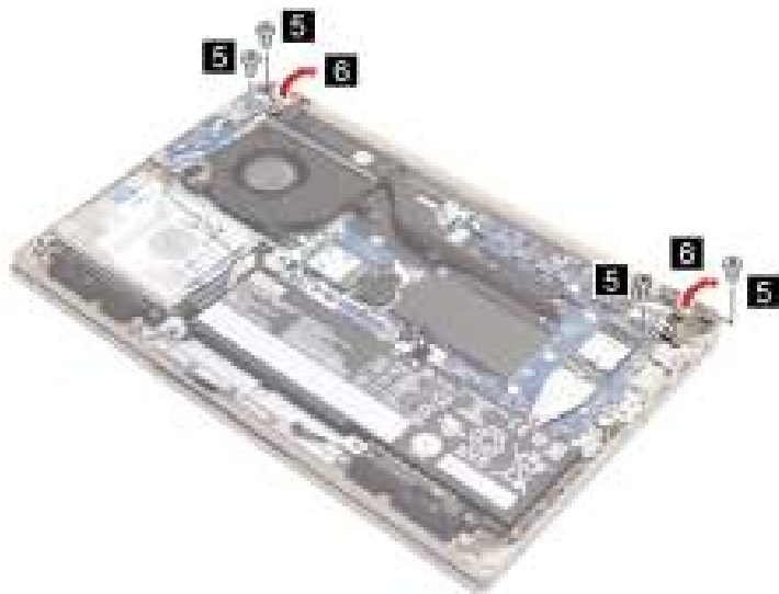
Figure 55. Remove four screws and open both hinges
