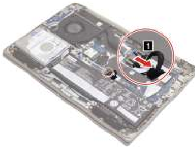
Figure 15. Disconnect the battery pack cable
