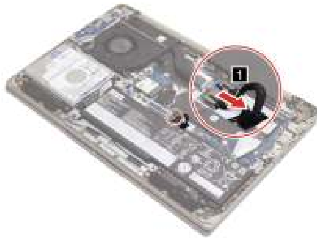
Figure 41. Disconnect the battery pack cable
