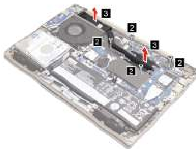
Figure 24. Loosen four screws and remove the heat sink
