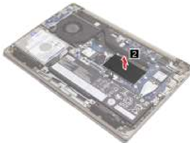
Figure 10. Remove the memory module shielding
