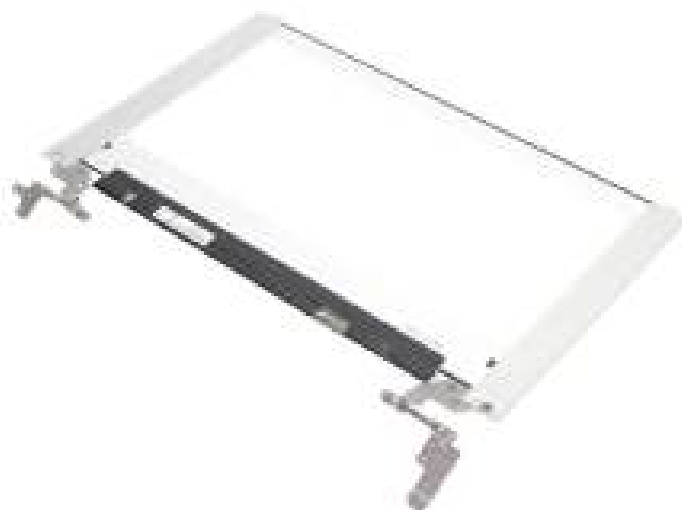
Figure 67. Remove the LCD assembly
