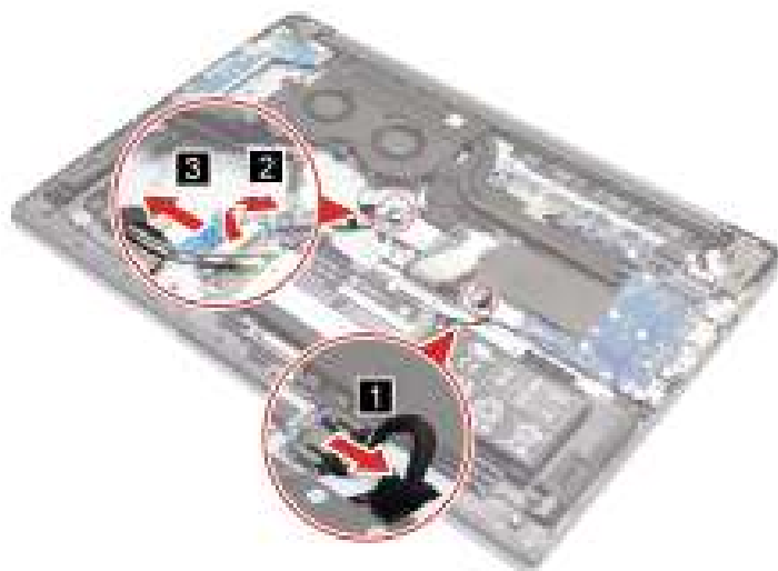
Figure 38. Disconnect the battery pack and the USB board cable
