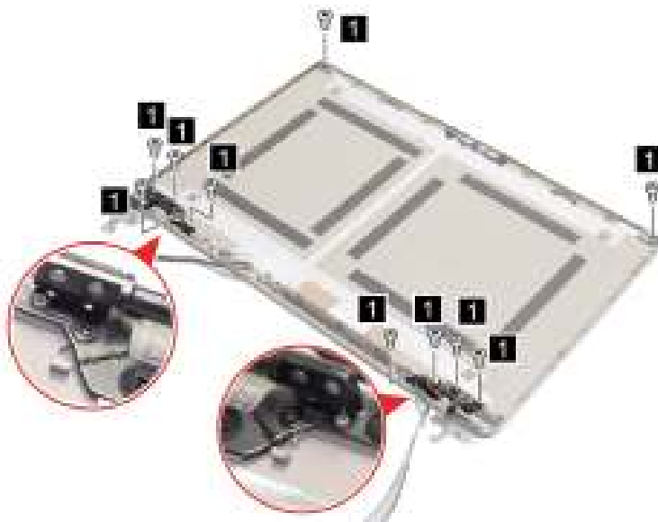
Figure 59. Remove ten screws
