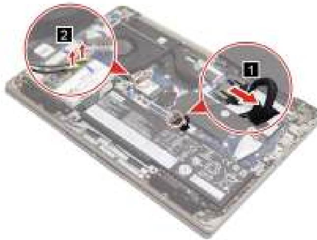
Figure 32. Disconnect the battery pack and Wi-Fi card cable
