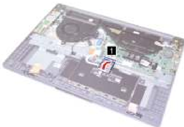
Figure 32. Peel back the keyboard cable
