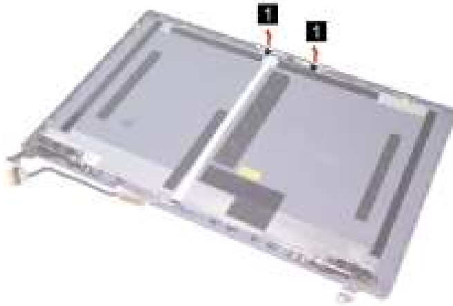
Figure 60. Remove the microphone rubbers
