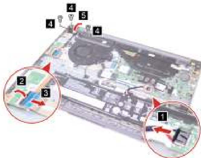
Figure 29. Disconnect the battery pack cable and I/O board cable, remove three screws and lift the left hinge
