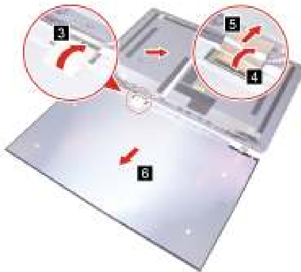
Figure 56. Disconnect the EDP cable and remove the LCD panel
