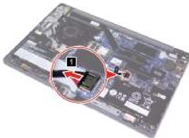
Figure 9. Disconnect the battery pack cable
