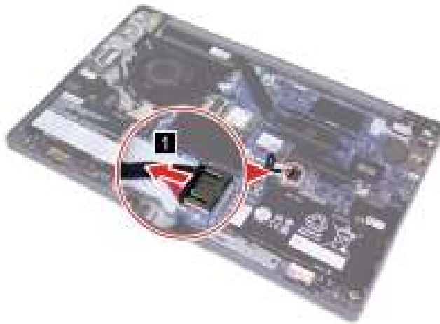
Figure 27. Disconnect the battery pack cable
