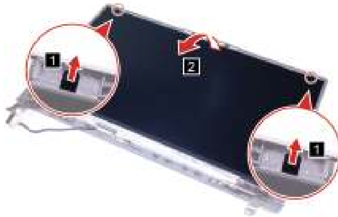
Figure 55. Remove the LCD panel
