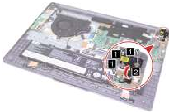
Figure 45. Remove three screws and lift the right hinge
