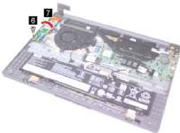
Figure 30. Remove one screw and remove the I/O board
