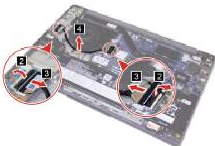
Figure 25. Disconnect and remove the I/O board cable
