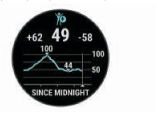
3 Press **DOWN** to view a combined graph of your Body Battery and stress levels.
