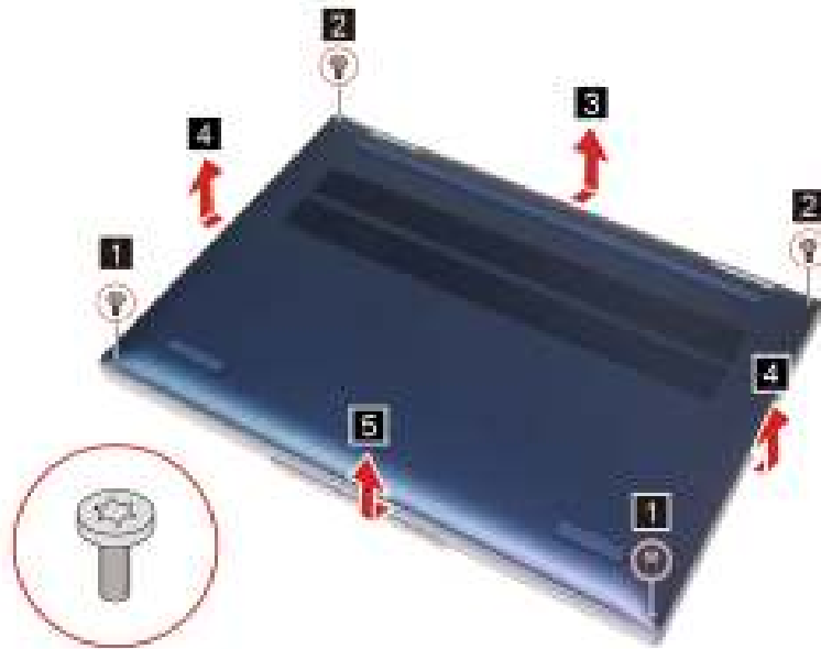
Figure 4. Remove four screws and the lower case
