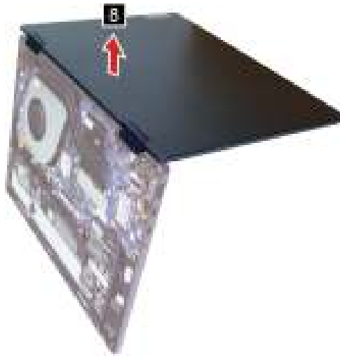
Figure 48. Rotate and remove the LCD module
