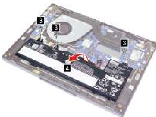
Figure 7. Remove three screws and the battery pack
