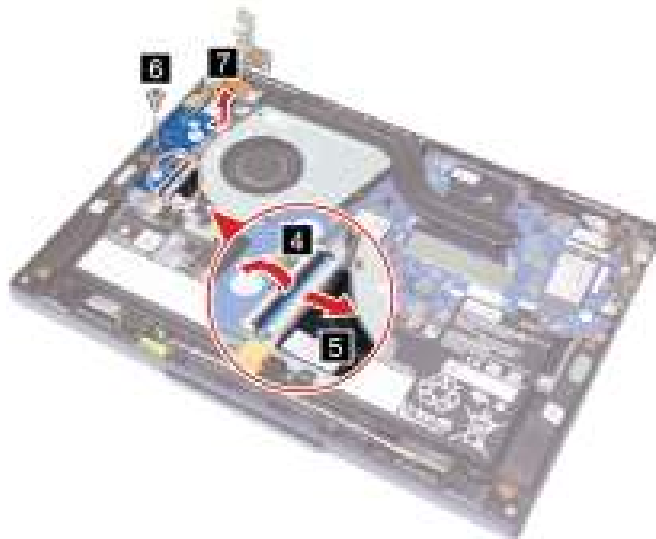
Figure 17. Disconnect the USB board cable, remove one screw, and remove the USB board
