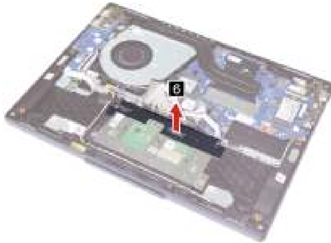
Figure 35. Remove the touchpad mylar
