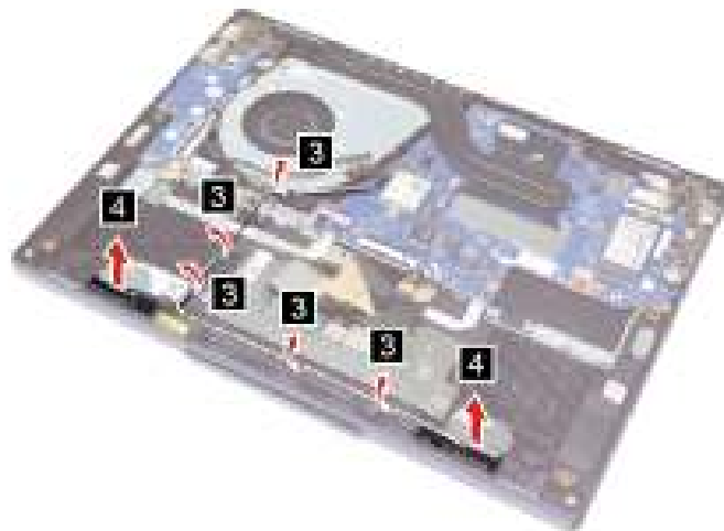
Figure 24. Remove the antennas
