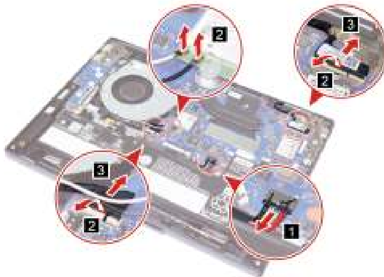
Figure 45. Disconnect the cables
