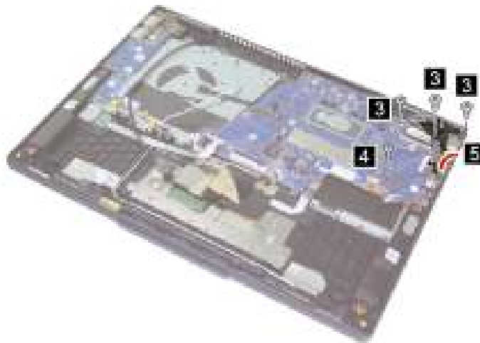
Figure 38. Remove four screws and open the right hinge
