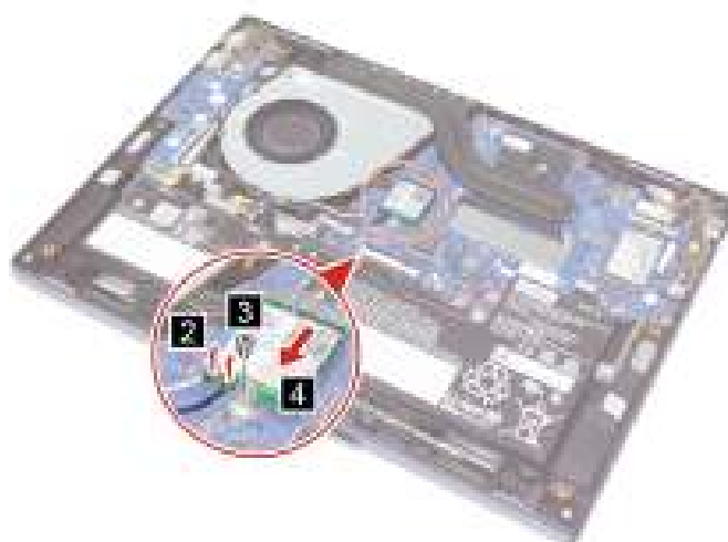
Figure 9. Disconnect the antennas, remove one screw and the Wi-Fi card
