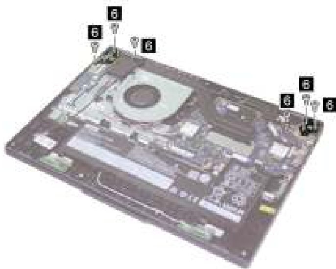
Figure 50. Remove six screws
