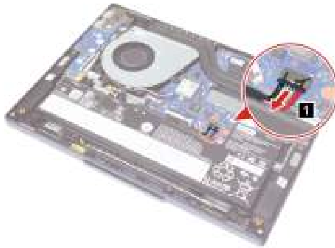
Figure 19. Disconnect the battery pack cable from the system board
