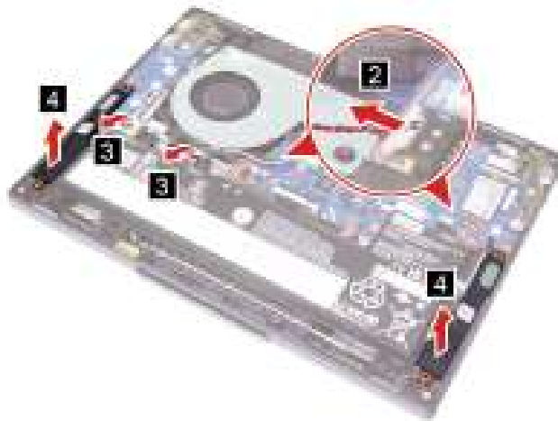
Figure 20. Disconnect the speakers cable and remove the speakers
