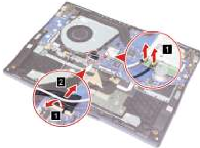
Figure 23. Disconnect the antennas and camera board cable
