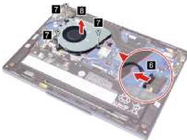
Figure 15. Disconnect the fan cable, remove three screws, and remove the fan
