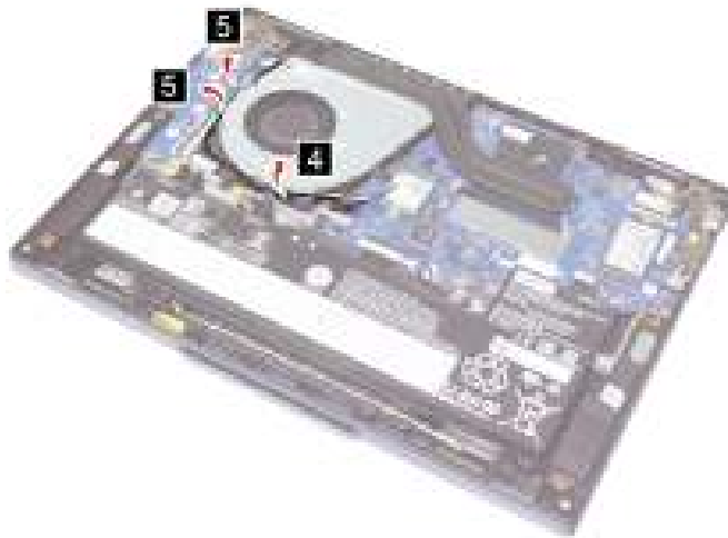
Figure 14. Remove the antennas and camera board cable from the cable guide
