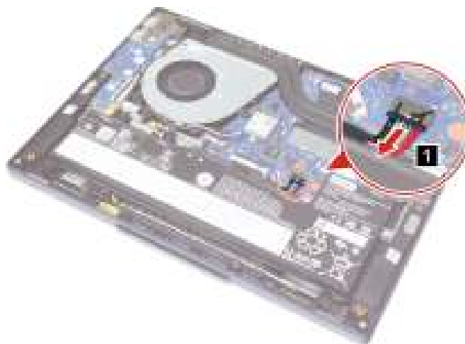
Figure 8. Disconnect the battery pack cable from the system board
