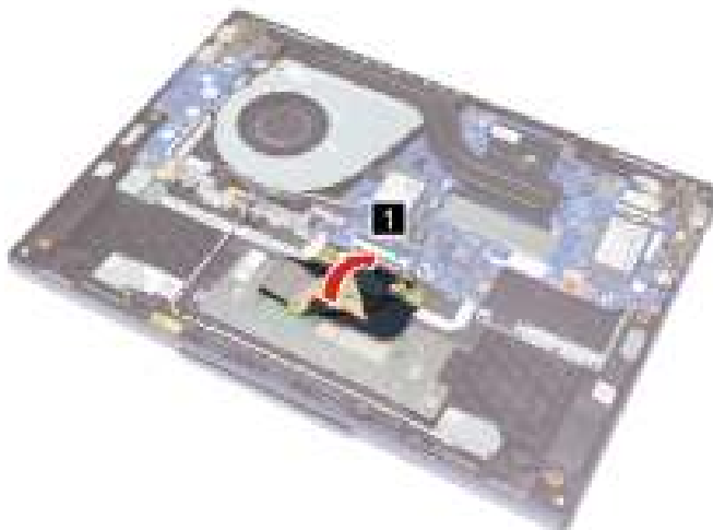
Figure 31. Peel back the keyboard cable
