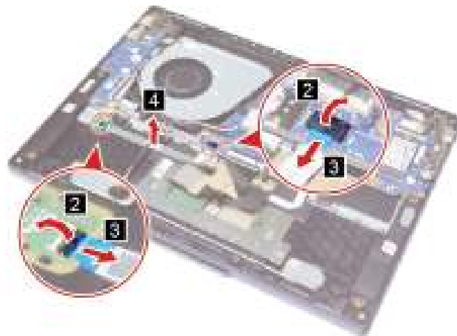
Figure 28. Disconnect and remove the fingerprint cable
