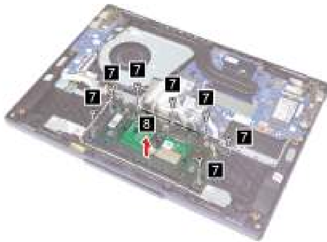
Figure 36. Remove seven screws and the touchpad
