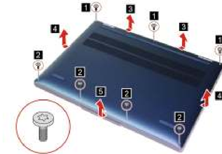
Figure 5. Remove seven screws and the lower case
