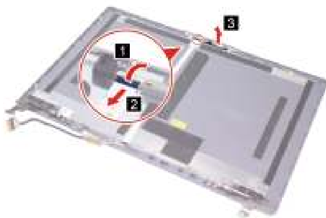
Figure 61. Disconnect the EDP cable and remove the camera board
