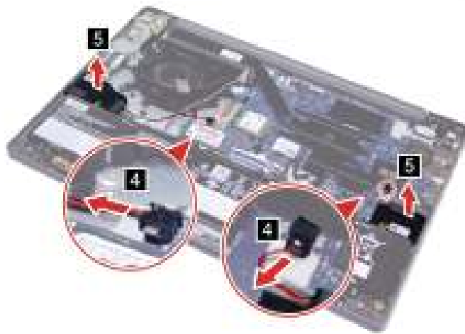
Figure 22. Disconnect and remove the speakers
