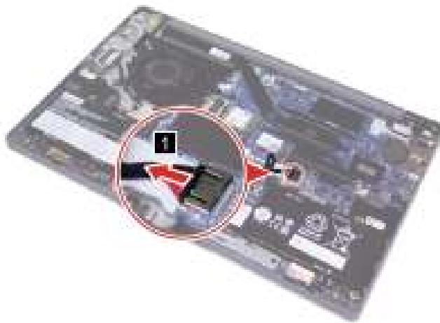
Figure 15. Disconnect the battery pack cable
