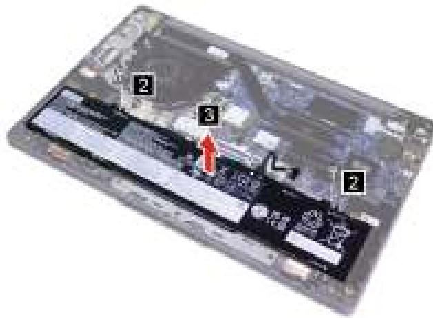
Figure 6. Remove the battery pack
