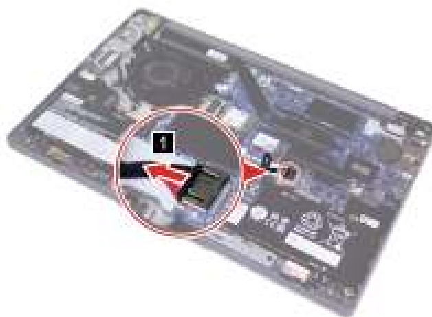
Figure 9. Disconnect the battery pack cable
