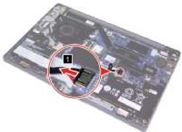
Figure 12. Disconnect the battery pack cable
