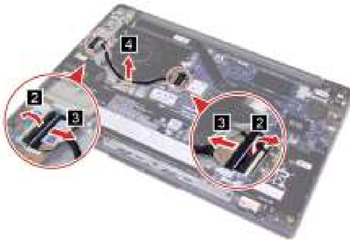
Figure 25. Disconnect and remove the I/O board cable
