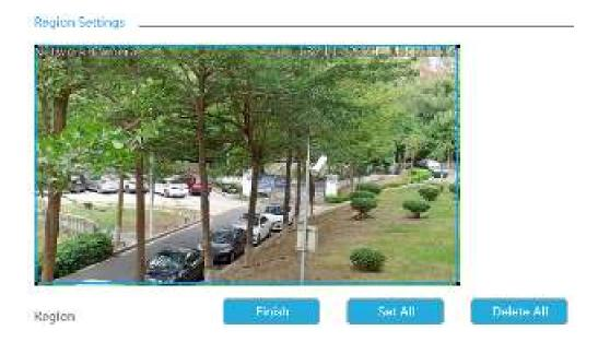
For cameras with the firmware version higher than 4X.7.0.78, it supports drawing polygon detection region for VCA function.
