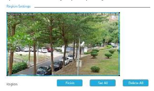
For cameras with the firmware version higher than 4X.7.0.78, it supports drawing polygon detection region for VCA function.
