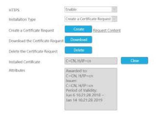
After creating and installing the certificate successfully, you can check the certificate information and clear the information on the following interface. And you can access the NVR by inputting <a href="https://ip:port">https://ip:port</a> via the web browser.
