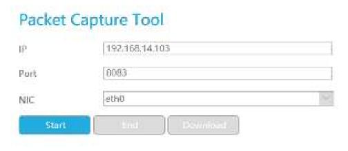
Note: It is recommended to capture packets not more than 3 minutes on the local monitor side.
