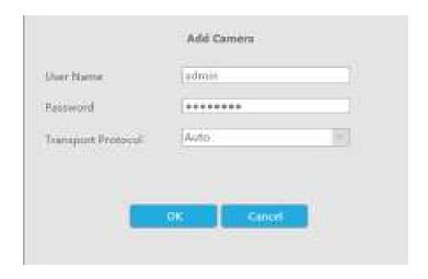
Method 2. Add camera through camera management interface. 'Camera'→'Camera Management'.
