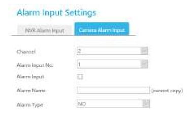
**Alarm Input No.:** The channel which has input signal.
