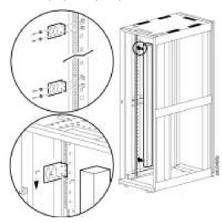
Route the power cable out of the rack and connect it to an appropriately rated branch circuit of your power source. The Rack PDU should be connected to a dedicated circuit protected by a branch circuit breaker that matches the Rack PDU input-plug type. Turn the power feed circuit breaker ON.
