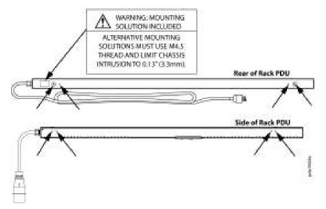
Two (2) Rack PDUs can be installed on one (1) vertical accessory channel in a NetShelter rack.
