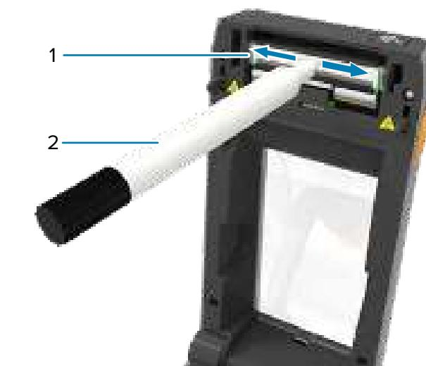
Clean printhead (1) with a cleaning pen (2). Clean from the middle to the outside. The cleaning pen is only for cleaning a printhead.
