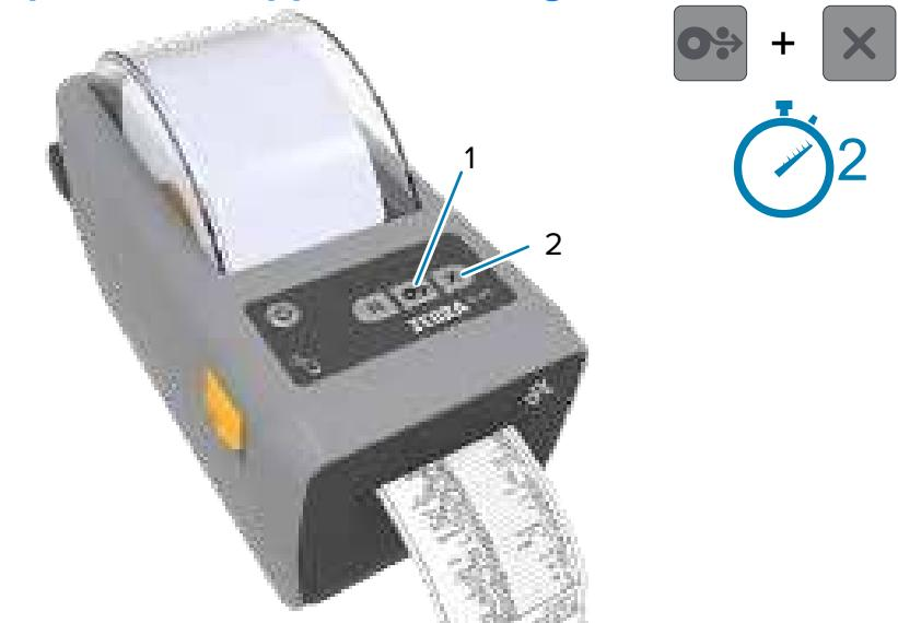
Press and hold the Feed (1) and Cancel (2) buttons for two seconds to print a configuration report.
