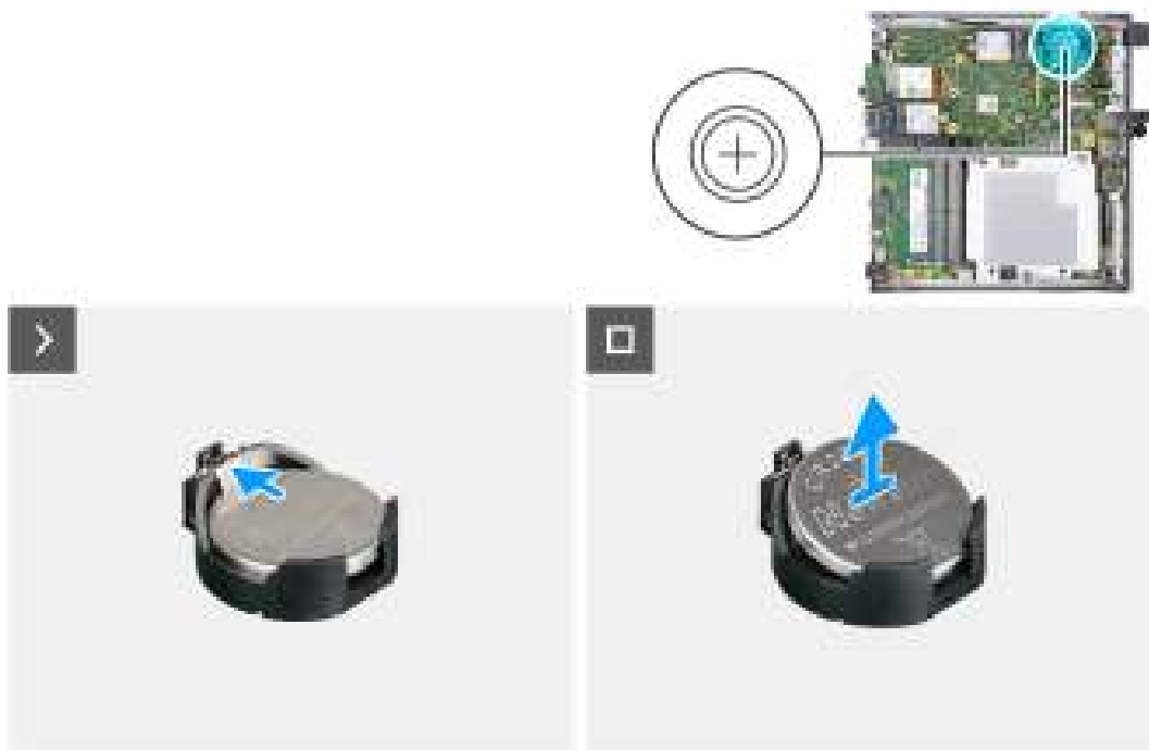
Figure 13. Removing the coin-cell battery
