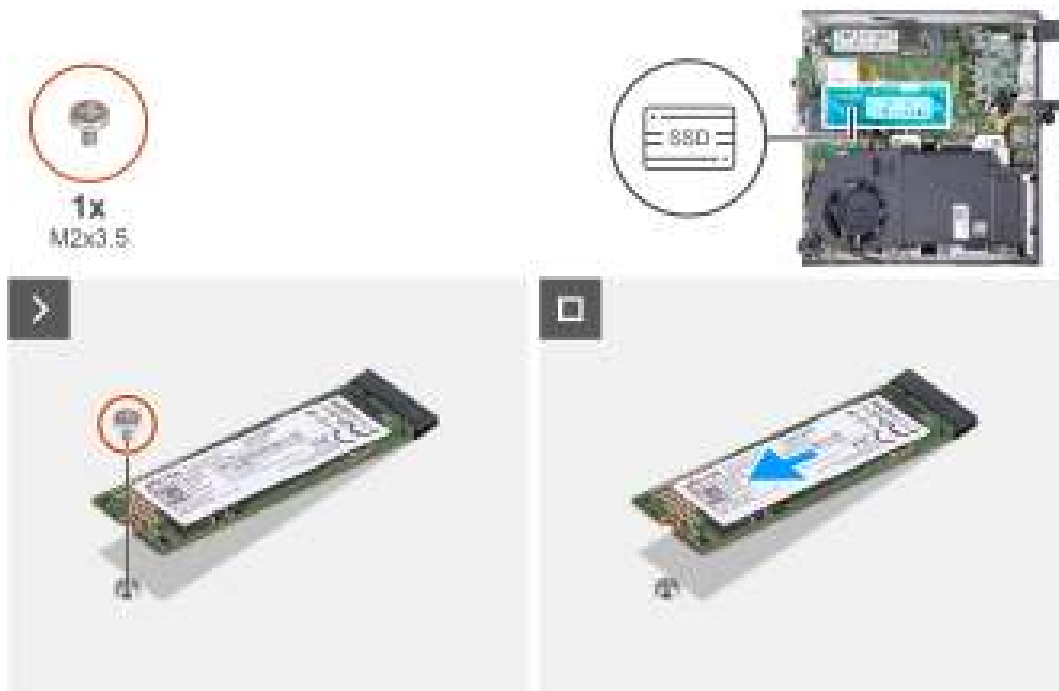
Figure 21. Removing the M.2 2280 solid-state drive from slot 0
