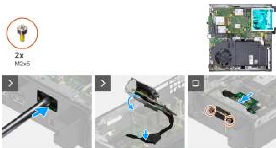
Figure 37. Installing optional I/O module (VGA or Serial)
