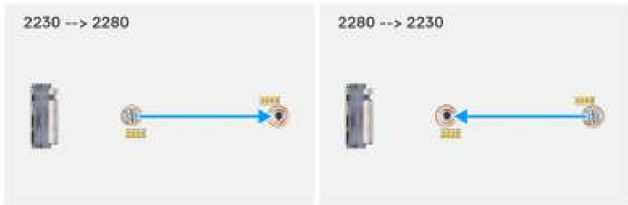
Figure 27. Moving the screw mount to support a different form factor (OptiPlex Micro 7020)
