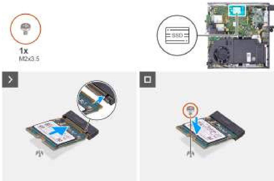
Figure 24. Installing the M.2 2230 solid-state drive in slot 1
