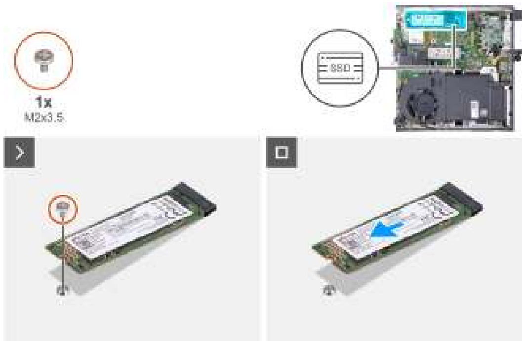
Figure 25. Removing the M.2 2280 solid-state drive from slot 1
