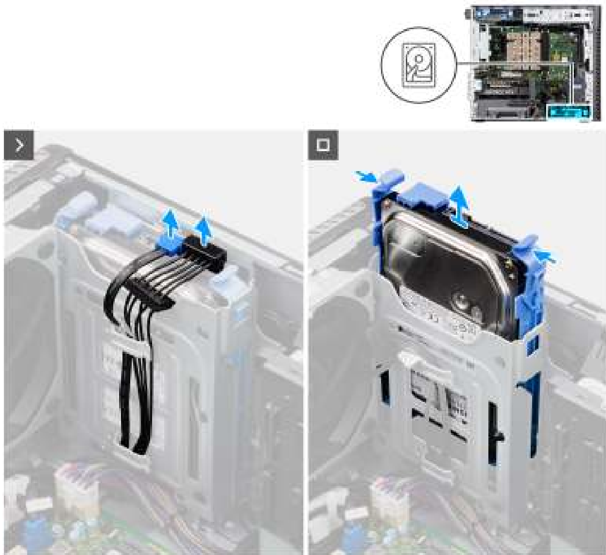
Figure 16. Removing the 3.5-inch hard drive assembly from Bay 1
