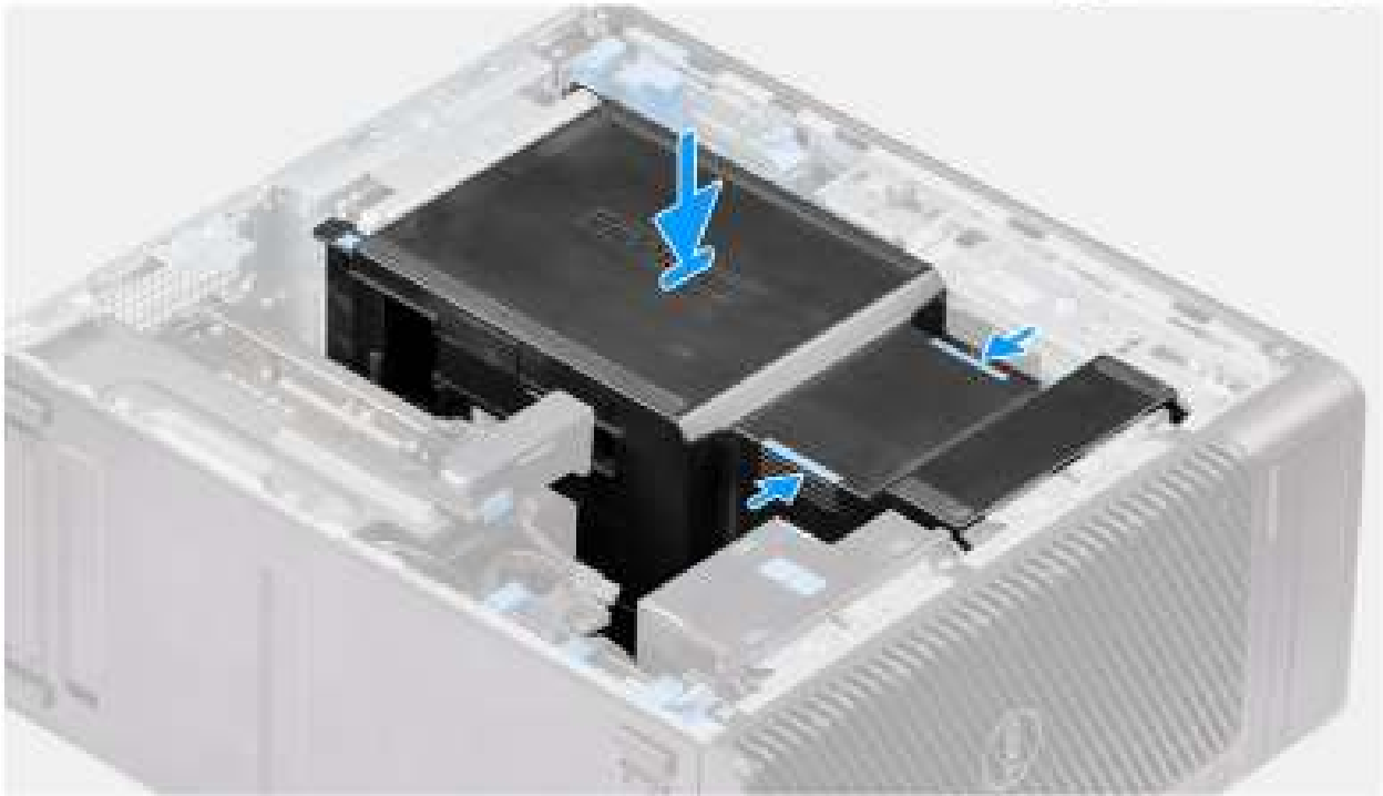
Figure 15. Installing the air shroud
