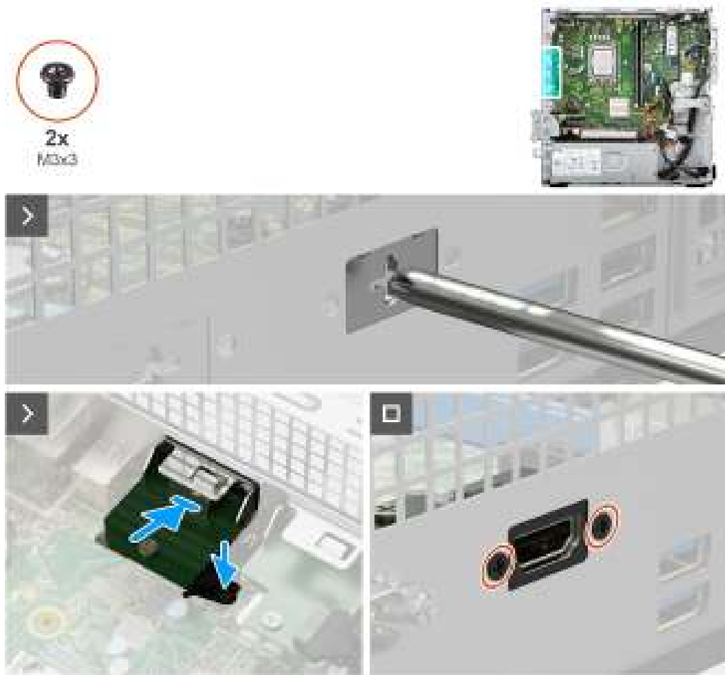
Figure 55. Installing the HDMI module
