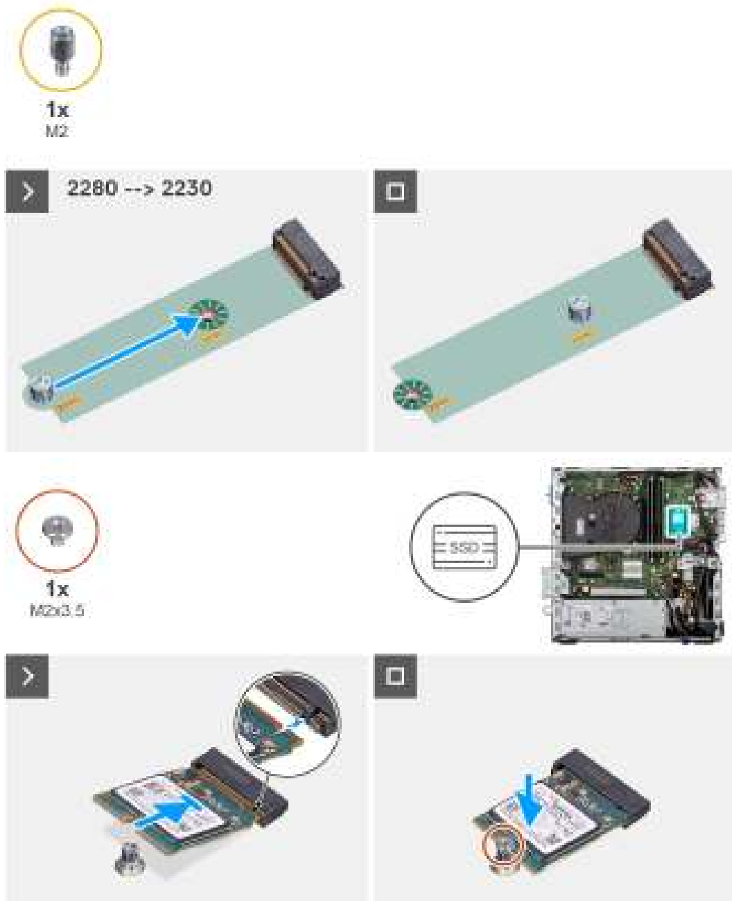
Figure 18. Installing the M.2 2230 solid-state drives
