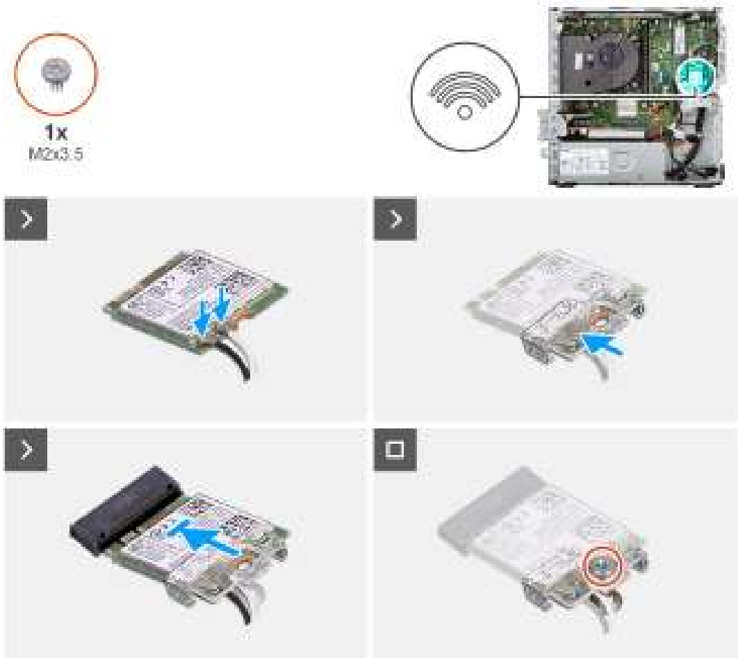
Figure 28. Installing the wireless card
