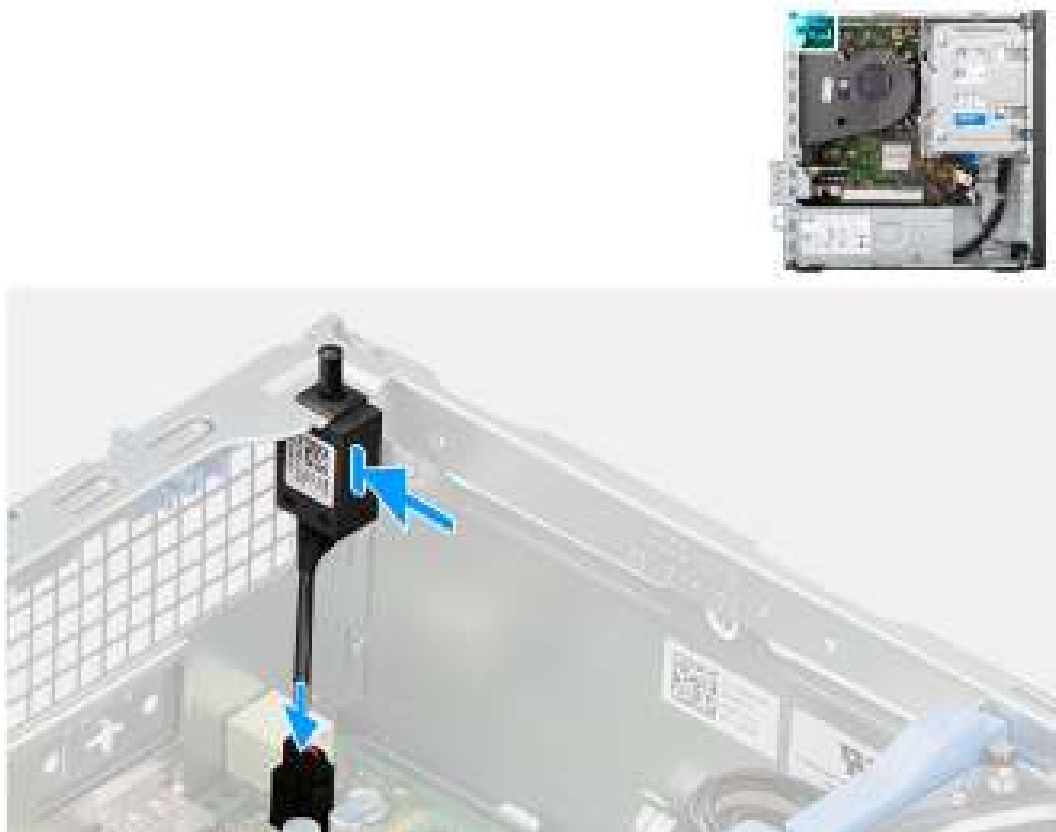
Figure 34. Installing the Intrusion switch
