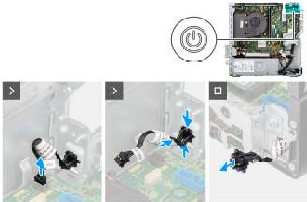
Figure 35. Removing the power button
