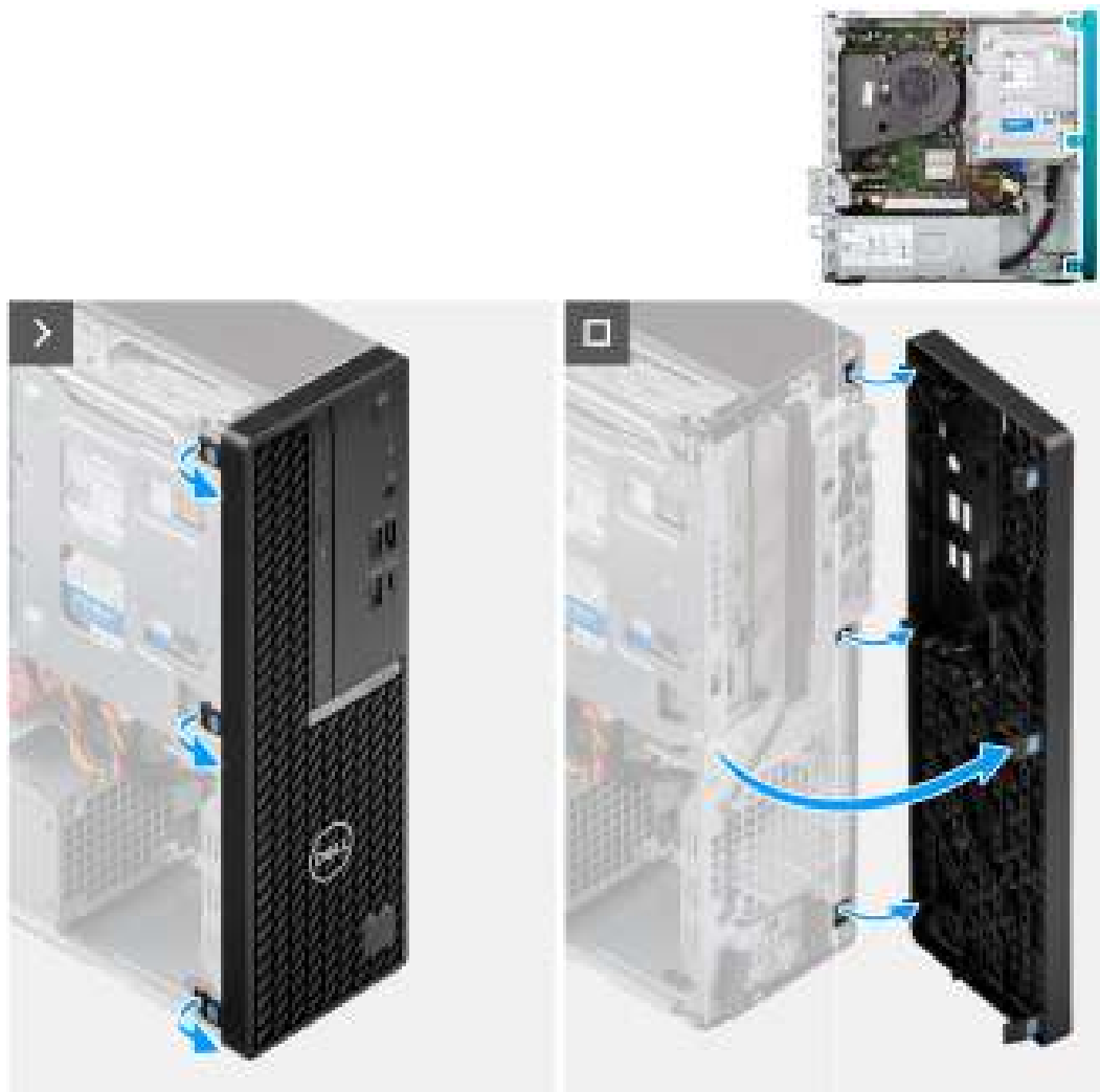
Figure 7. Removing the front bezel
