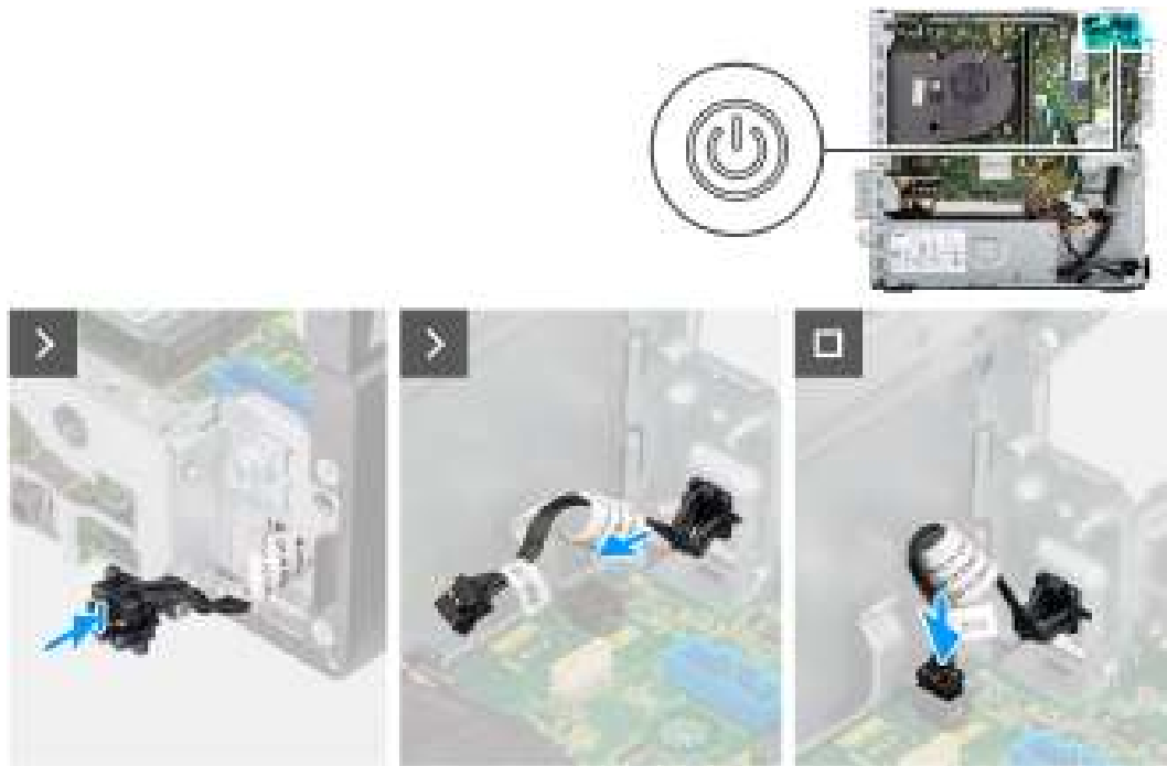
Figure 36. Installing the power button
