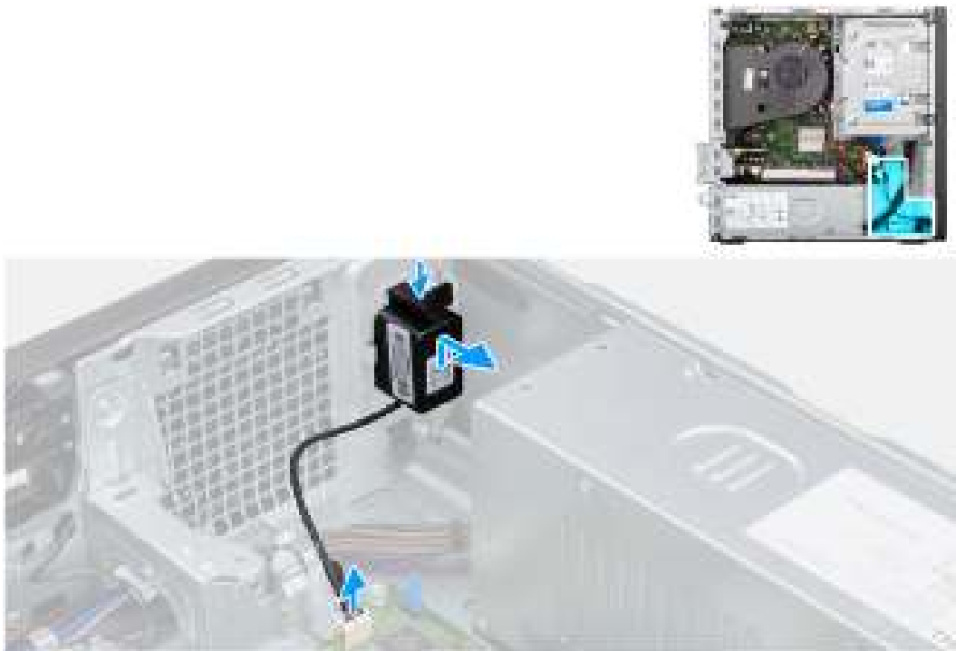
Figure 31. Removing the speaker
