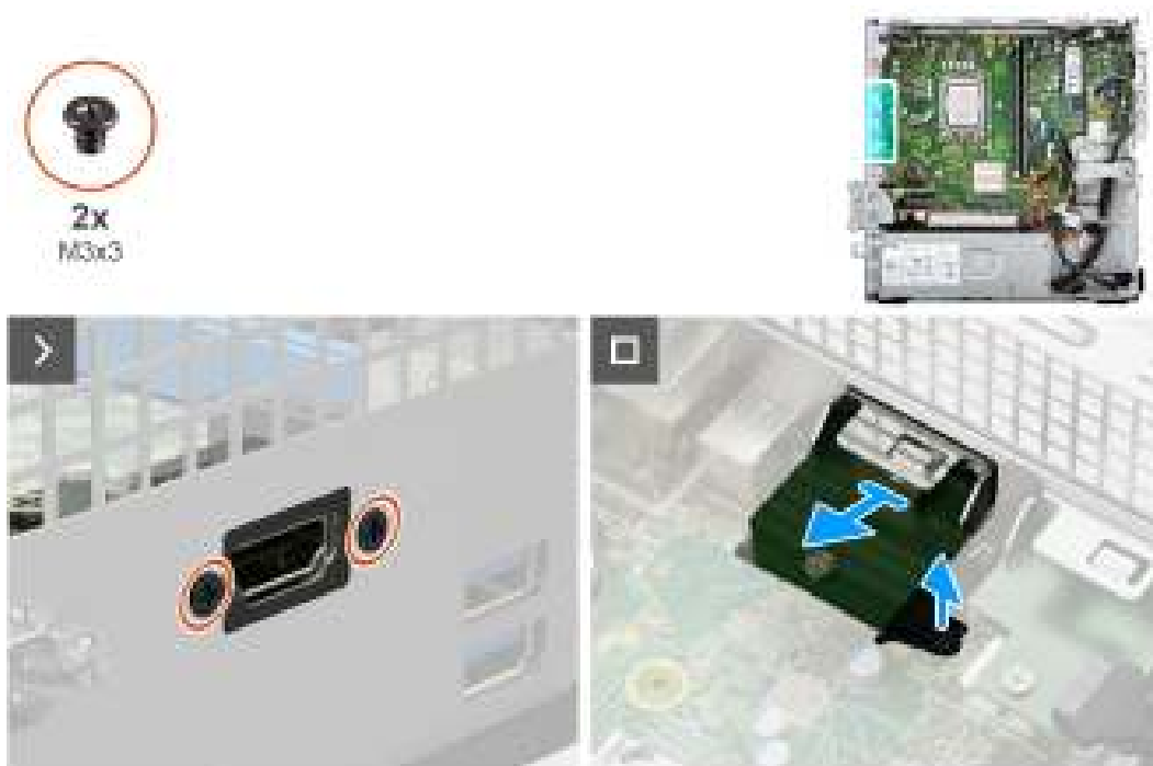
Figure 54. Removing the HDMI module
