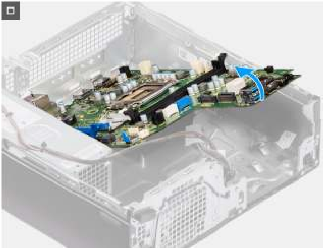
Figure 60. Removing the system board
