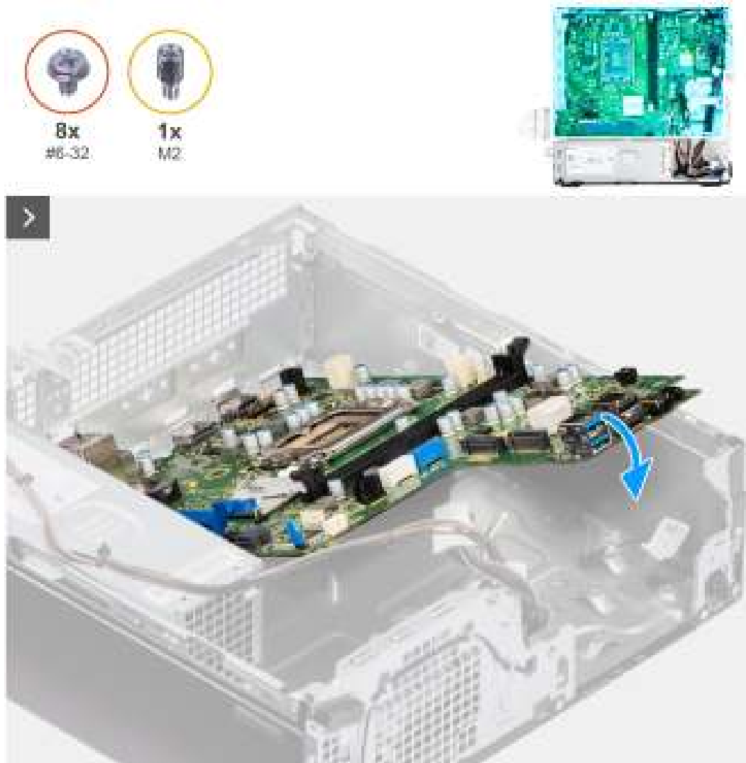
Figure 62. Installing the system board
