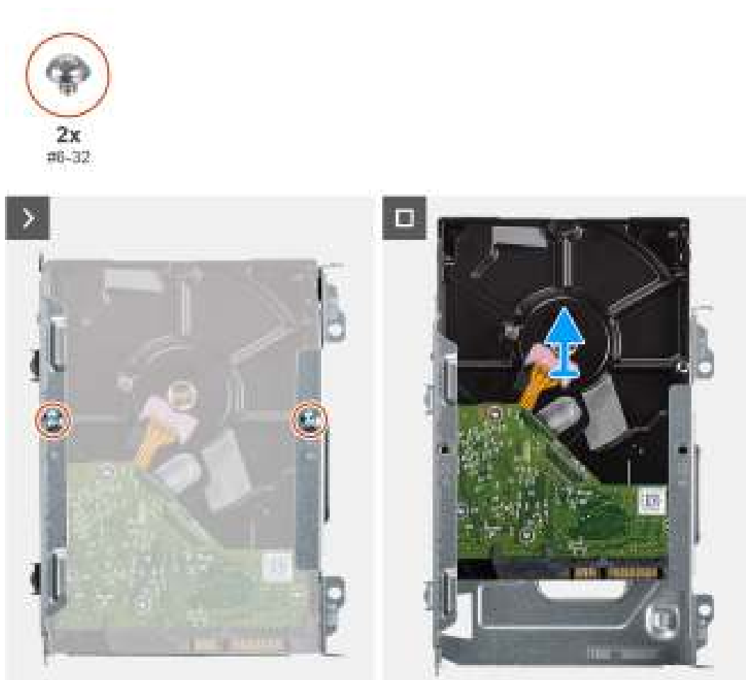
Figure 9. Removing the 3.5-inch hard drive
