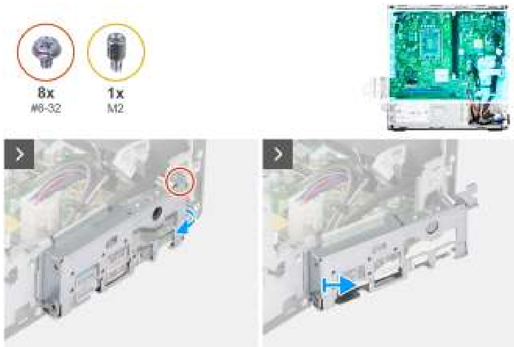
Figure 57. Removing the system board
