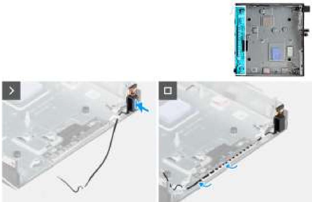
Figure 53. Installing the antenna module (black cable)
