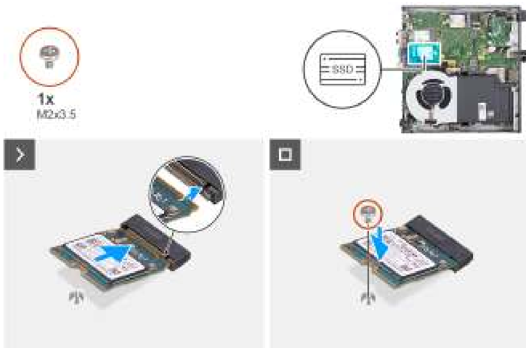
Figure 20. Installing the 2230 solid-state drive in slot 0
