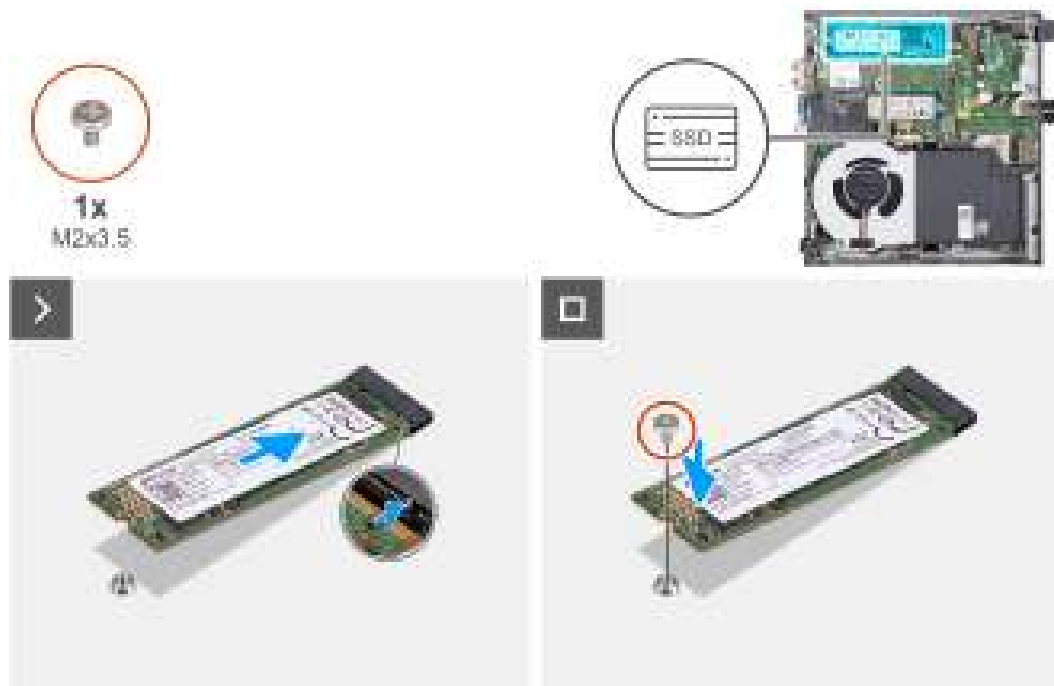
Figure 26. Installing the M.2 2280 solid-state drive in slot 1
