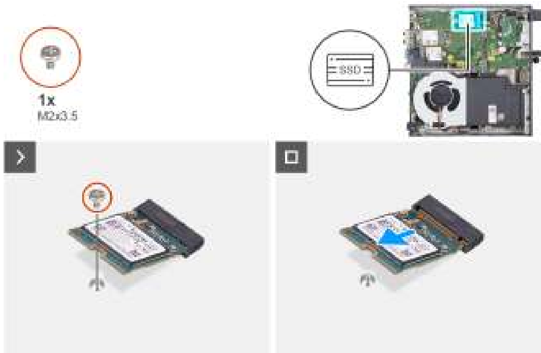
Figure 21. Removing the M.2 2230 solid-state drive from slot 1
