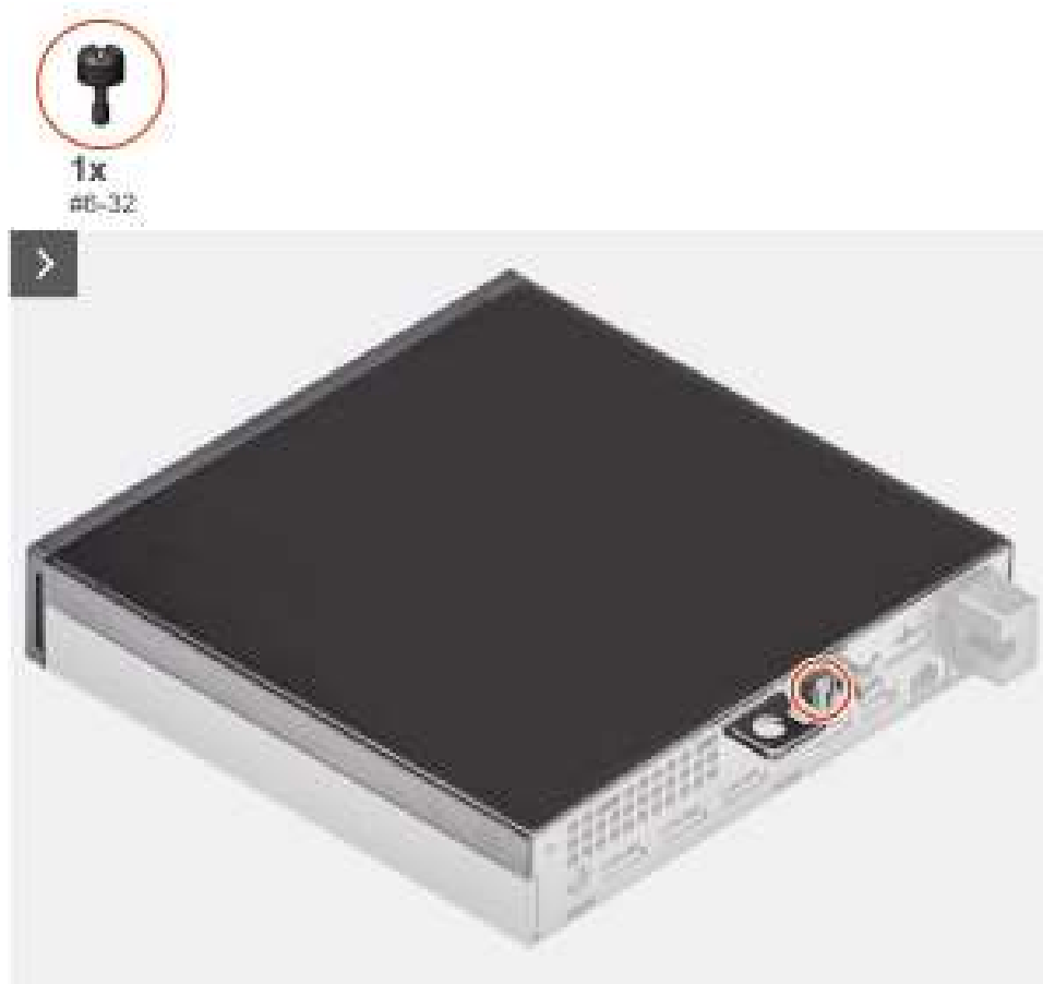
Figure 9. Removing the side cover
