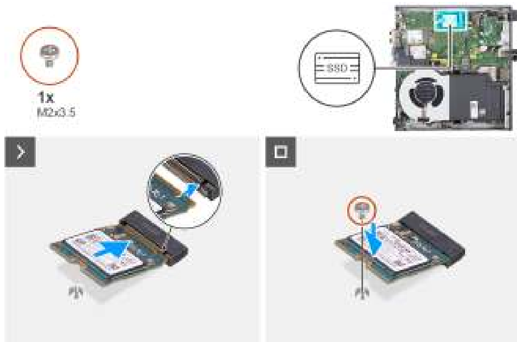
Figure 22. Installing the M.2 2230 solid-state drive in slot 1
