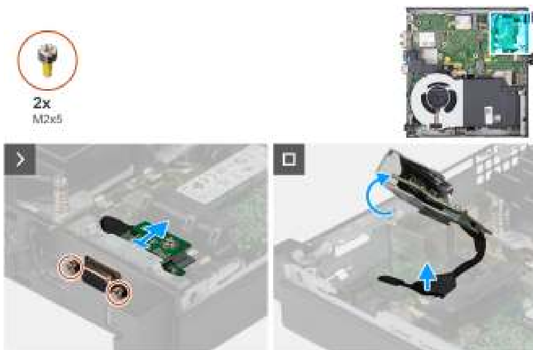
Figure 35. Removing the optional I/O module (VGA or Serial)
