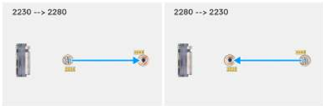
Figure 27. Moving the screw mount to support a different form factor (OptiPlex Micro Plus 7020)
