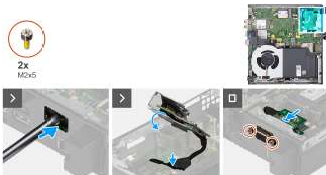
Figure 37. Installing optional I/O module (VGA or Serial)
