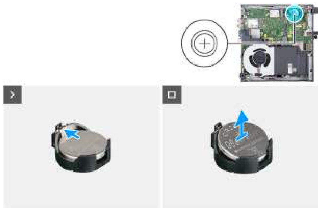
Figure 13. Removing the coin-cell battery
