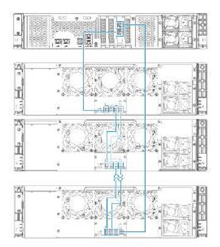
**2.** Connect the expansion units to the device using the following topology.
