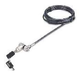
The Universal Laptop Lock is a versatile solution compatible with Noble Wedge, K-Slot (T-Bar), or Nano, providing flexibility and convenience. Its on-the-fly lock tip adjustment feature enables effortless compatibility with the different security slot types. The cut-resistant steel security cable measures 6.5 ft (2 m) in length and 0.17 in (4.4 mm) thick, providing reach and durability. With the 3-in-1 Laptop Lock, protect your valuable devices wherever you go.
