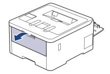
4. Use both hands to slide the manual feed slot paper guides to fit the width of the envelope that you are using.
