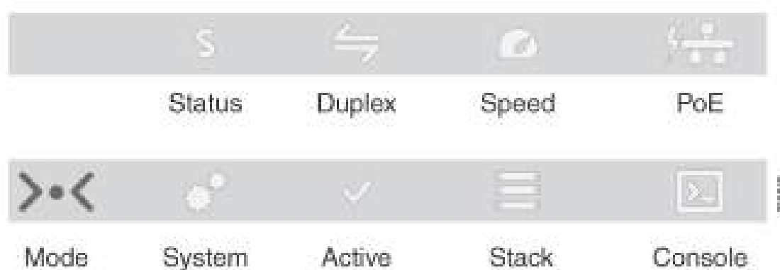
Figure 35: Switch Front Panel LEDs
