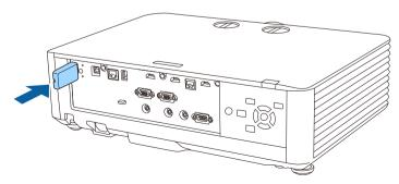
Attach the cover comes with your wireless LAN module, and secure it in place with the screw.
