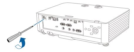
**2** Connect the wireless LAN module to the USB-A port.
