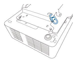
Attach the wire clamp to another carabiner, and then use the screw to fix the wire clamp to the wire clamp fixing point on the projector.
