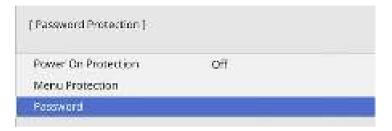
If you do not see this menu, hold down the [Freeze] button on the remote control for 5 seconds until the menu appears.
