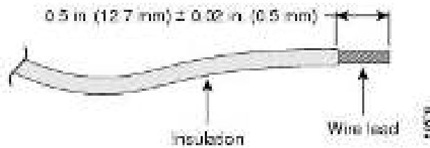
Figure 41: Stripping the Ground Wire
