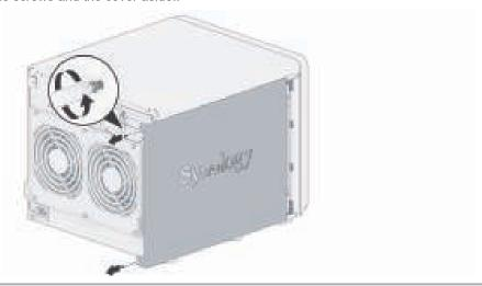
**Note:** When you remove the cover, sensitive internal components are exposed. Avoid touching anything other than the memory assembly when removing or adding memory.
