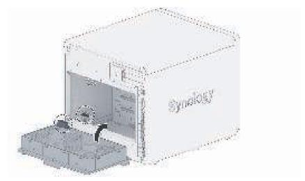
**b** Make sure that all 6 push pins on the new module are pulled outwards before the module is placed into your Synology NAS, and then press the push pins back into place to secure the fan module.
