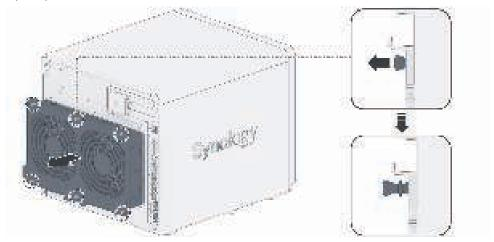
4 Pull out the malfunctioning fan module to remove it from your Synology NAS.
