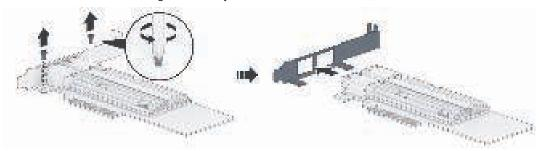
2 Replace the long bracket with a short one, and tighten the 2 screws to secure the short bracket.
