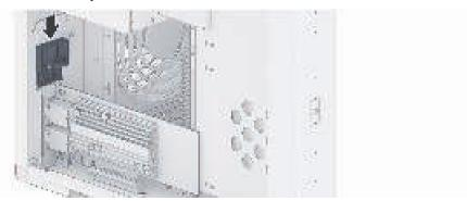
**Note:** Confirm that the connector is fully inserted. Otherwise, the network interface card might not be able to function properly.
