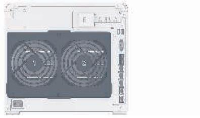
3 Pull the 6 push pins that secure the fan module.
