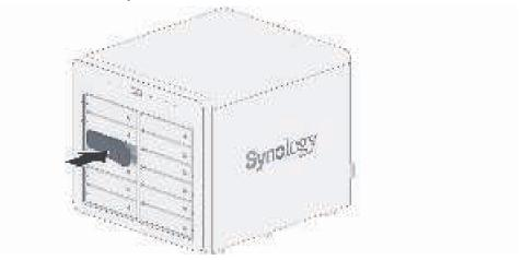
2 Pull out the hard drive tray handle as shown below to remove the hard drive tray.
