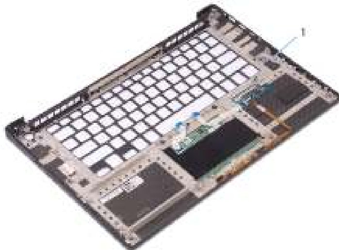
Figure 36. Removing the palm-rest assembly
