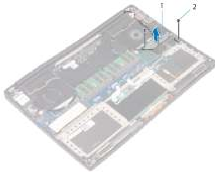
Figure 19. Removing the display-cable bracket
