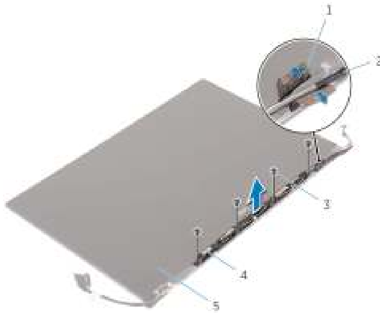
Figure 35. Removing the antenna module
