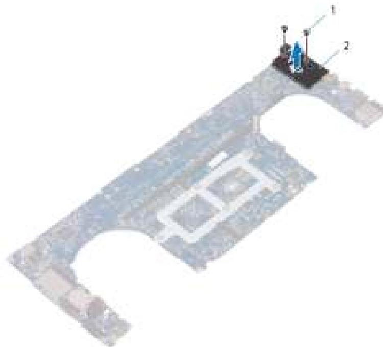
Figure 24. Removing the audio daughter-board
