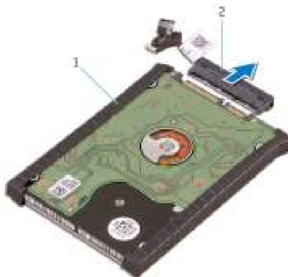
Figure 9. Disconnecting the hard-drive interposer from the hard-drive assembly
