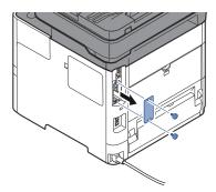
3 Insert the SD/SDHC memory card into the SD/SDHC memory card slot.
