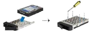
• For 2.5" drives: Place the drive in the drive tray. Turn the tray upside down and tighten screws into the four spots indicated below to secure the drive in place.
