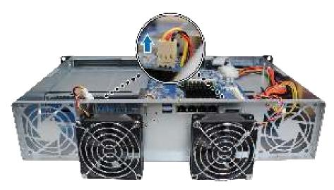
**b** Remove the screws that secure the fan guard from the malfunctioning fan.
