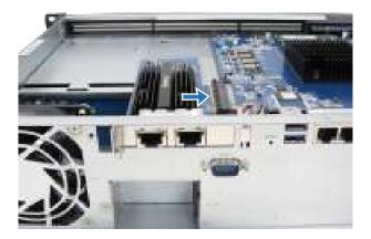
c Place back the latch and fasten the screw that you removed in step 2-a to secure the newly inserted card in place.
