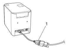
1 RJ25 to DB9M serial adapter
