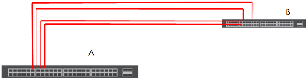
Figure 125 Trunking Example - Physical Connections
