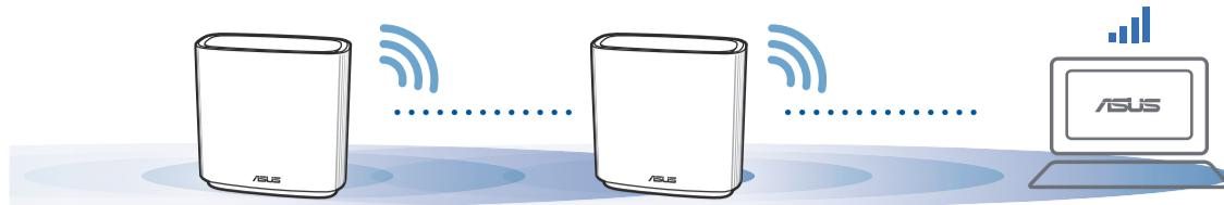
**NOTES:** To minimize interference, keep the routers away from devices like cordless phones, Bluetooth devices and microwave ovens. We recommend that you place the routers in an open or spacious location.
