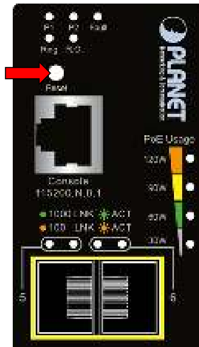
Figure 2-9 IGS-5225-4P2S Reset Button
