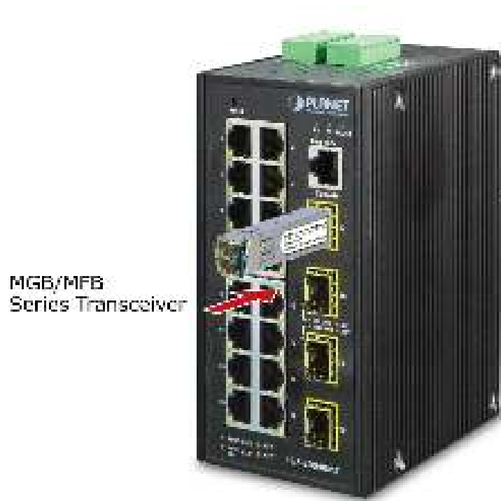
Figure 2-19: Plugging in the SFP/SFP+ Transceiver
