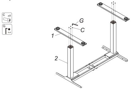
• Connect the feet (1) and the lifting column (2) with screws (C) and tighten them with the allen key (G)
