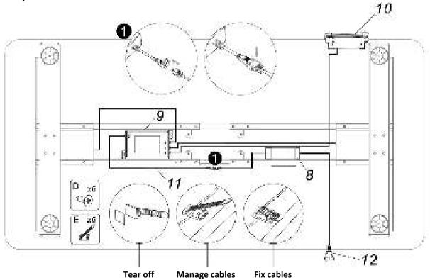
Fix the cables to the tabletop with cable management (E), and then use screw (D) to fix the cable management (E) to keep the desk cables organized.
