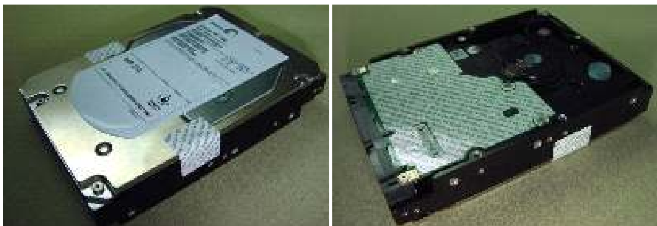
Figure 11. Example of FIPS tamper evidence labels.
