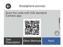
5. On your iPhone, iPad or iPod touch, start the standard Camera app, and then scan the QR code displayed on the printer's control panel in PHOTO mode.
