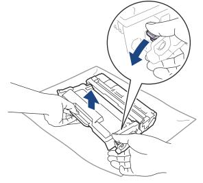
9. Turn the drum unit as shown in the illustration. Make sure that the drum unit gear (1) is on the left side.
