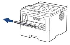
4. Slide the MP tray paper guides to fit the width of the paper you are using.
