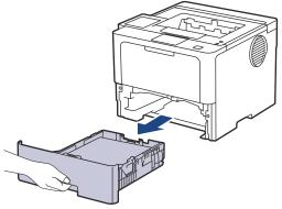
3. At the back of the machine, pull the 2-sided tray completely out of the machine.
