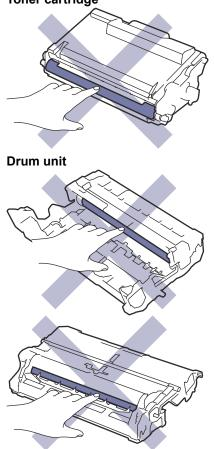
Both the toner cartridge and the drum unit feature an IC chip. DO NOT touch these surfaces. Touching the IC chips may cause contamination or damage, and may interfere with the machine's ability to detect these components.
