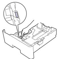
5. Wipe the two pick-up rollers inside the machine to remove dust.
