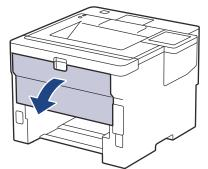
7. Pull the green levers at the left and right sides towards you to release the fuser cover.
