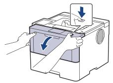
3. Remove the toner cartridge and drum unit assembly from the machine.
