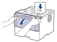
3. Remove the toner cartridge and drum unit assembly.
