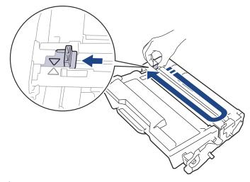
Be sure to return the tab to the Home position (**A**). The arrow on the tab must be aligned with the arrow on the drum unit. If it is not, printed pages may have a vertical stripe.
