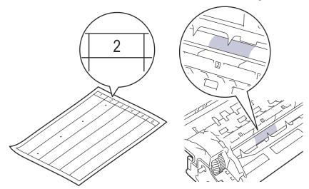
11. Turn the drum unit edge towards you while looking at the drum surface to find the mark.
