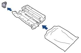
7. Push the toner cartridge firmly into the new drum unit until it locks into place.
