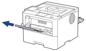
5. Slide the MP tray paper guides to fit the width of the envelopes that you are using.
