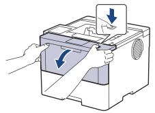
2. Remove the toner cartridge and drum unit assembly from the machine.
