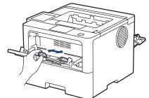
6. Load labels with the printing surface face up in the MP tray.
