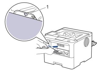
Load the envelopes in the MP tray with the printing surface face up. Make sure the envelopes are below the maximum paper mark (1).
