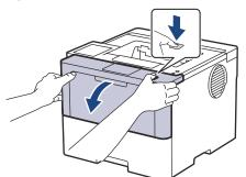
7. Remove the toner cartridge and drum unit assembly from the machine.
