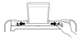
3. Load envelopes short edge first at the center of the paper support with the flap facing down.
