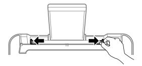
Load paper at the center of the paper support with the printable side facing up.
