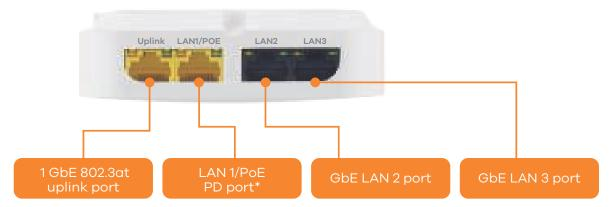
\*PoE PD port won't supply power (5 W) when the AP is powered by 30 W passive PoE injector.
