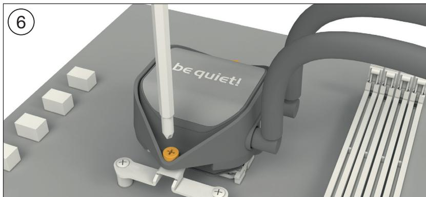
Place the CPU block centrally over the short AMD mounting brackets, such that these allow the CPU block to be screwed down. For this you can use a normal crosshead screwdriver. Next connect the pump and the ARGB illumination to the ARGB-PWM-Hub.
