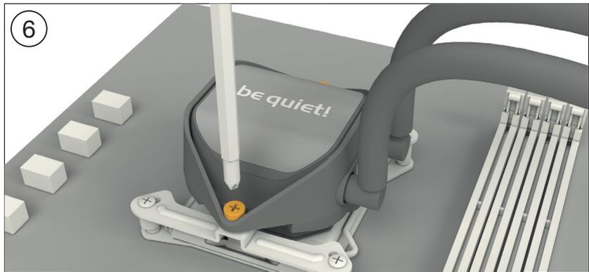
Place the CPU block centrally over the Intel mounting brackets, such that these allow the CPU block to be screwed down. For this you can use a normal crosshead screwdriver. Next connect the pump and the ARGB illumination to the ARGB-PWM-Hub.
