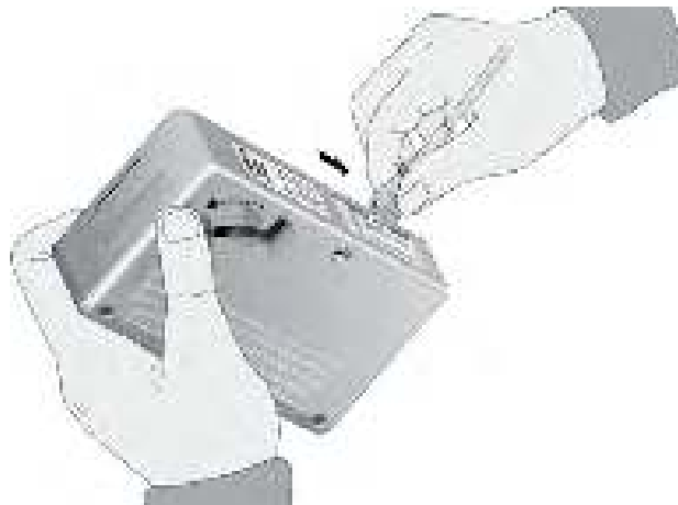
Figure 65. Rubbing the Ferrule Tip on the Cleaning Surface
