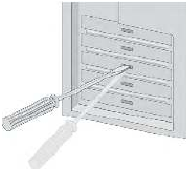
Figure 13. Removing the Faceplate From PCIe Slot
