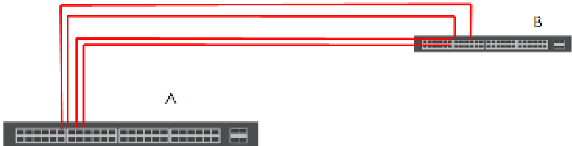
Figure 122 Trunking Example – Physical Connections
