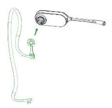
**2.** Choose the size of eartip that fits most comfortably. Align the eartip with the notch facing the microphone as shown. Press on to attach.
