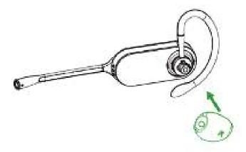
The earhook is flexible, and can be bent to suit your ear for a secure and comfortable fit.
