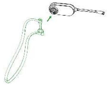
**4.** Choose the size of eartip that fits most comfortably. Align the eartip with the notch facing the microphone as shown. Press on to attach.
