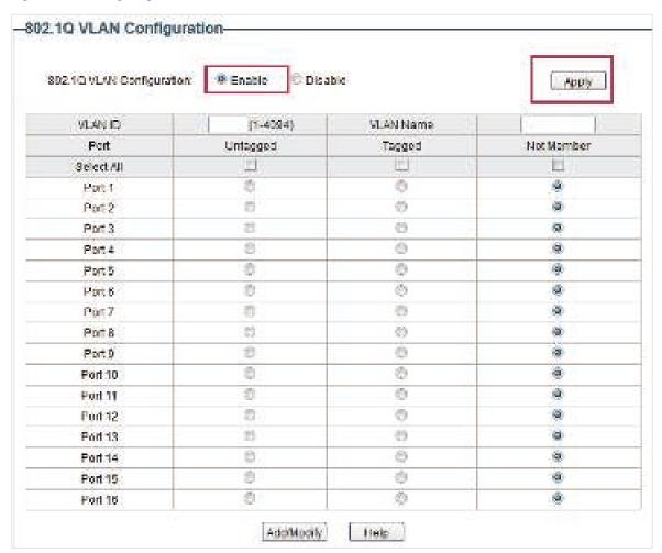
2) Choose the menu **VLAN > 802.1Q VLAN** to load the following page and create VLAN 2. Specify VLAN ID as **2**, add port 2 to the VLAN as an untagged port, and add port 4 to the VLAN as a tagged port. Click **Add/Modify**.
