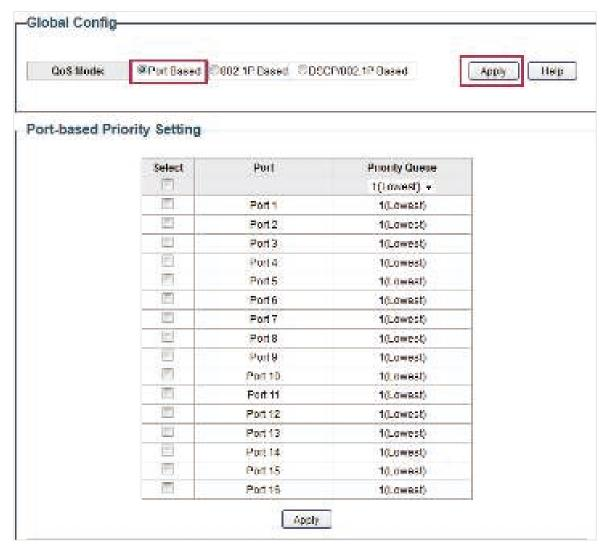
2) In the Port Based Priority Setting section, specify the priority queue for port 1 as 1(Lowest) and click Apply. Specify the priority queue for port 2 as 4(Highest) and click Apply.
