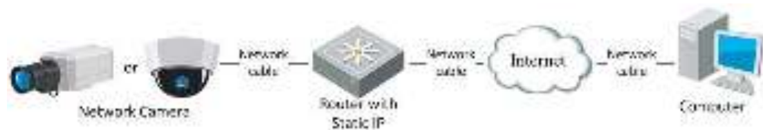
Figure 2-8 Accessing the Camera through Router with Static IP
