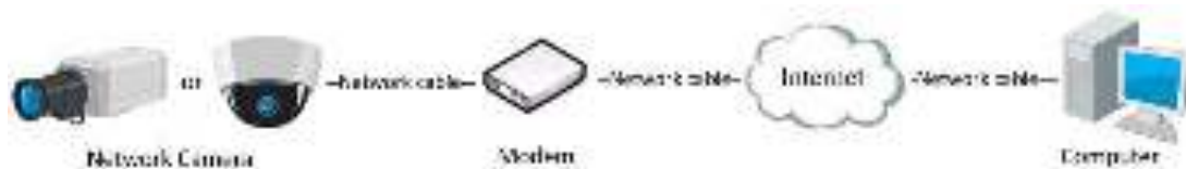
Figure 2-10 Accessing the Camera with Dynamic IP
