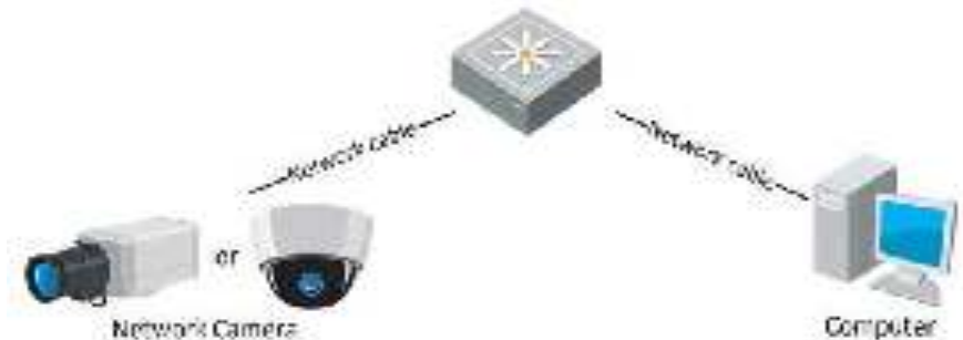
Figure 2-2 Connecting via a Switch or a Router
