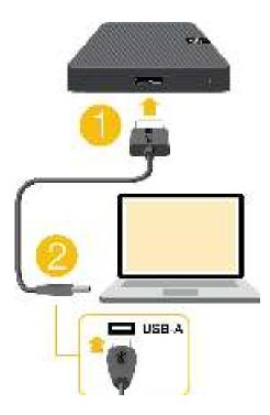
You can connect your Seagate device to a USB-C port on your computer. The USB-C port must support USB 3.0 or higher. A USB micro-B to USB-C cable is not included with this device.
