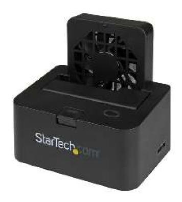
This USB 3.0 and eSATA docking station makes it easy for you to connect and swap your 2.5in or 3.5in SATA hard drives (HDD) and solid-state drives (SSD). The docking station also has a built-in fan that keeps your drives running at an optimal temperature for peak performance and longer drive lifespan.
