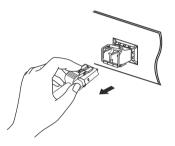
3. Pull the safety latch downwards to release the transceiver, and then pull it out from the slot.
