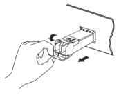
4. Reinstall the protective dust plug in the transceiver's optical bores and place it on antistatic mat or a static shielding bag.
