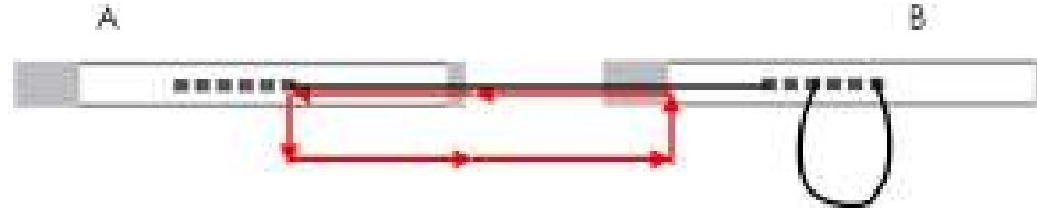
Figure 4 Two Connections between Switches without Spanning Tree Protocol (STP)
