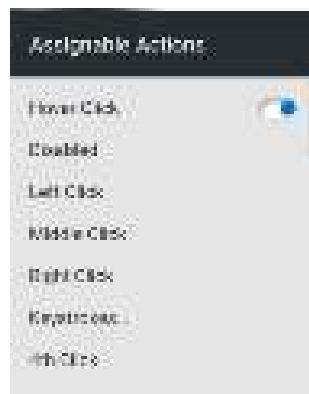
Of particular note is the "Hover Click" option, which enables the user to execute the action with the pen tip hovering near the screen instead of directly touching it.
