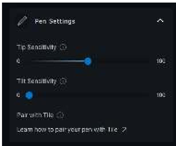
For supported applications such as Microsoft Whiteboard, the sensitivity settings will vary the brush width based on the amount of pressure and angle of the pen tip applied to the screen.
