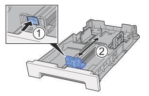
**3** Adjust the position of the paper width guides located on the left and right sides of the Cassette 2.
