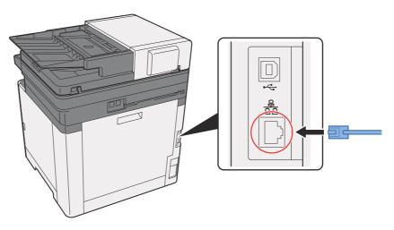
2 Connect the other end of the cable to the hub or the PC.
